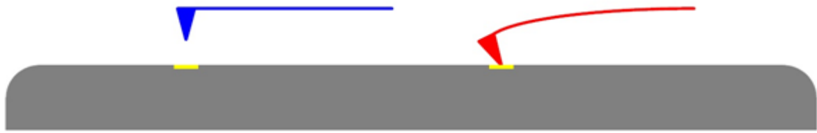
Figure 5.30: Different bending of the cantilever, because of different charging of the surface in the real system.
