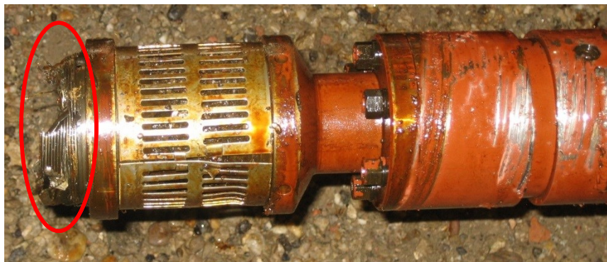
Figure 25: Intake/ gas anchor breakage [38]
