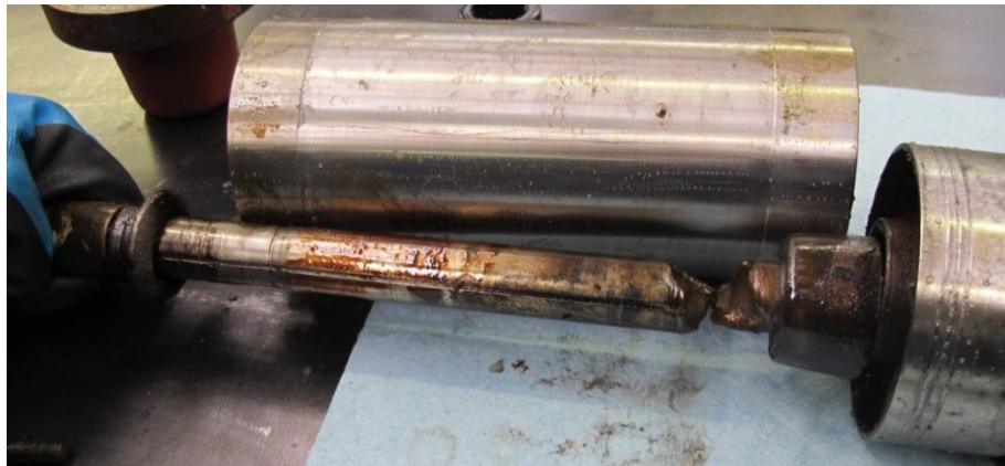
Figure 28: DIFA: broken shaft due to broken zirconium bearing [38]
