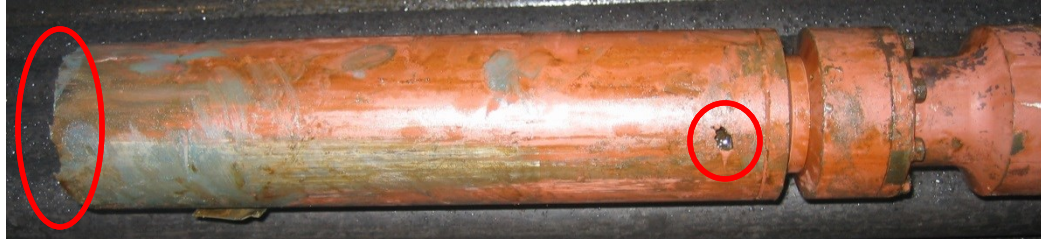
Figure 23: Broken pump/ leakage of housing [38]
