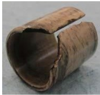
Figure 27: DIFA broken zirconium bearing [38]
