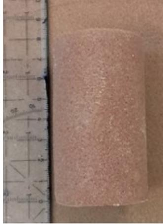
Figure 6: Core plug drilled from outcrop Bentheim Sandstone
