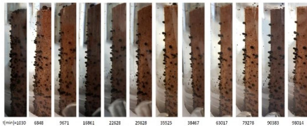
Figure 24: Droplets distribution on the plug's wall during the time for the system B8-H1-8TH-H1
