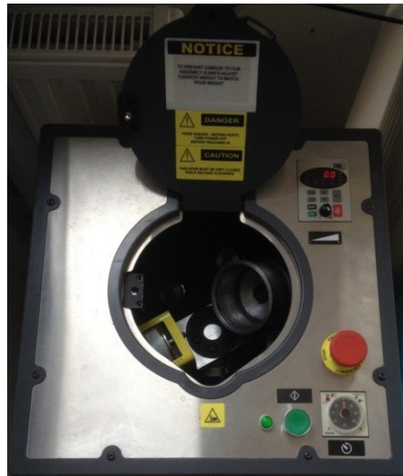
Figure 5-1 Vortex mixer VM-200 used for manufacturing of PU foam in laboratory
