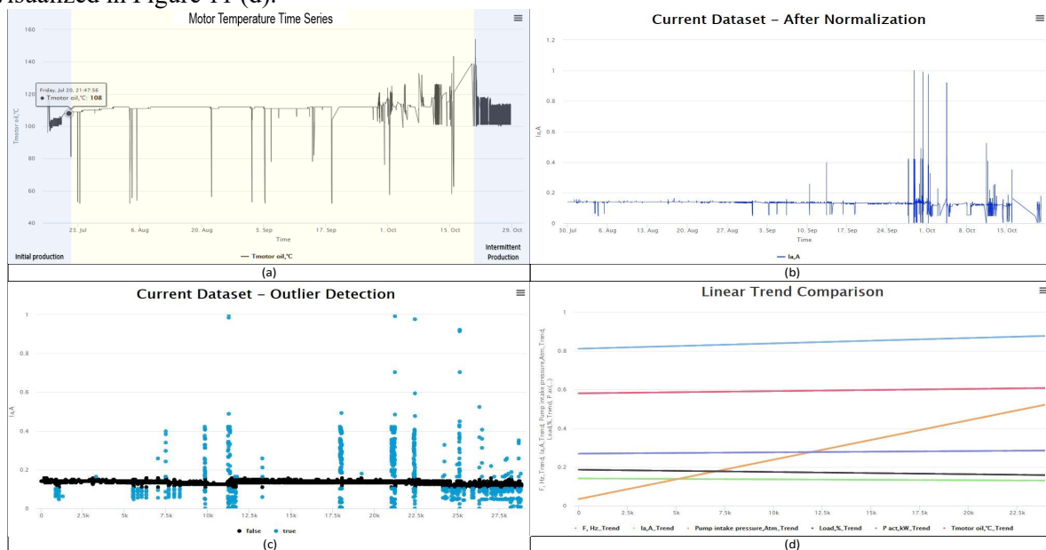
Figure 11. Trend extraction procedure; a – raw data; b – cleansed and filtered data; c – outlier detection; d – linear trends
