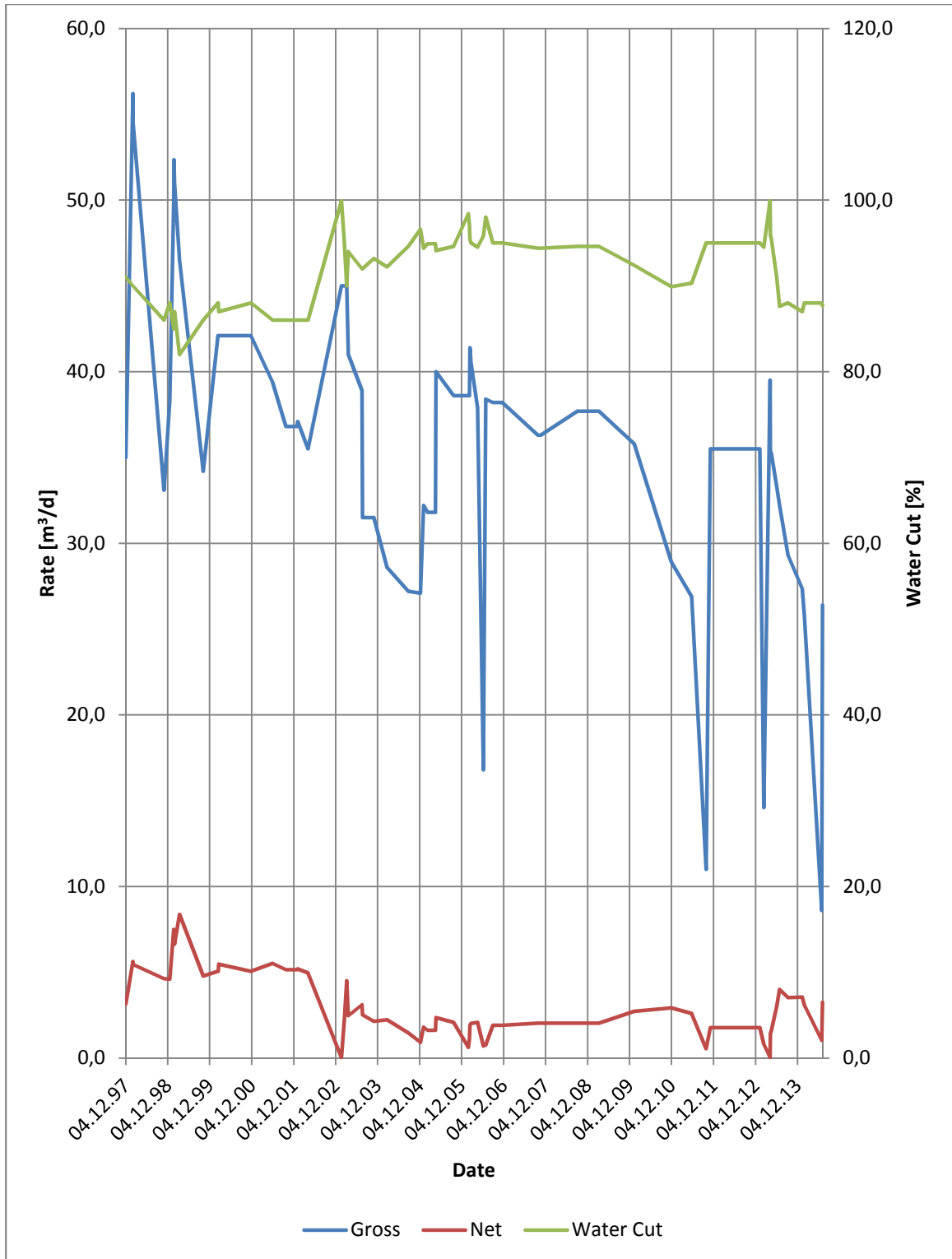
Figure 30: Production history of well PSI-006 located in the field Psi
