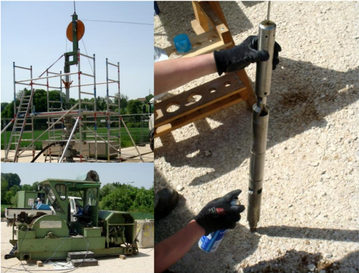
Figure 6: Left upper picture shows the deployment of the tool on a cap string. The left lower picture shows the capillary string unit. The right picture shows the Hydropuls® tool itself.
