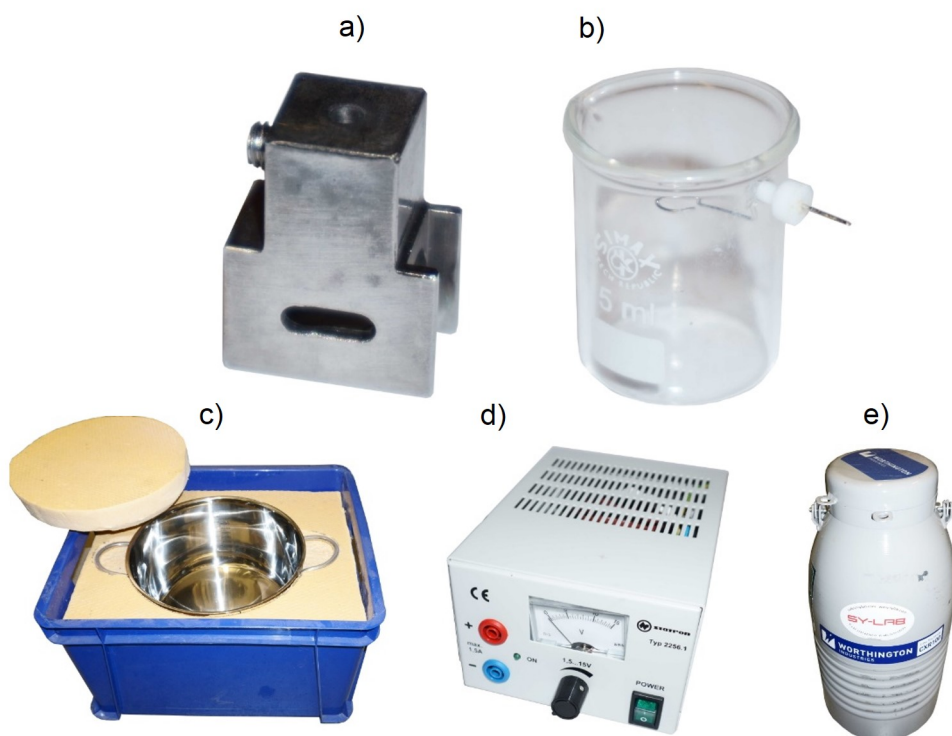
Figure 4.2: a) sample holder, b) beaker with Pt wire loop, c) isolated pot for LN 2 quenching, d) laboratory power supply, e) LN 2 transport dewar.
