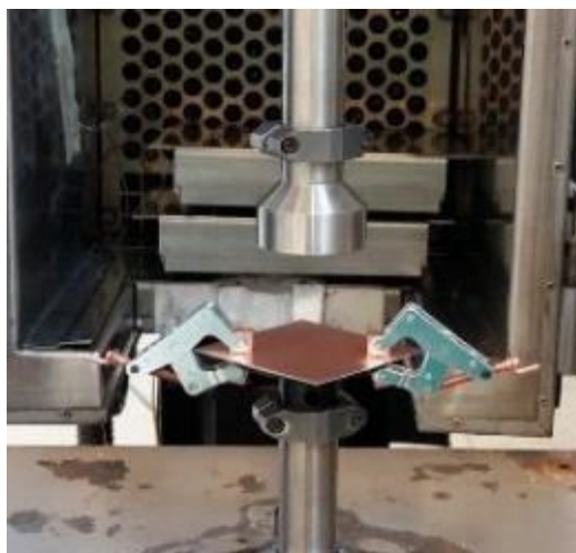
Figure 25: Experimental Set-up of surface tack measurements
