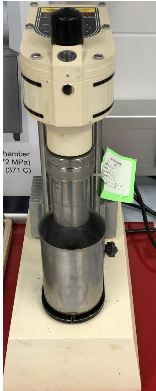
Figure 42: Chandler viscometer 3500M
