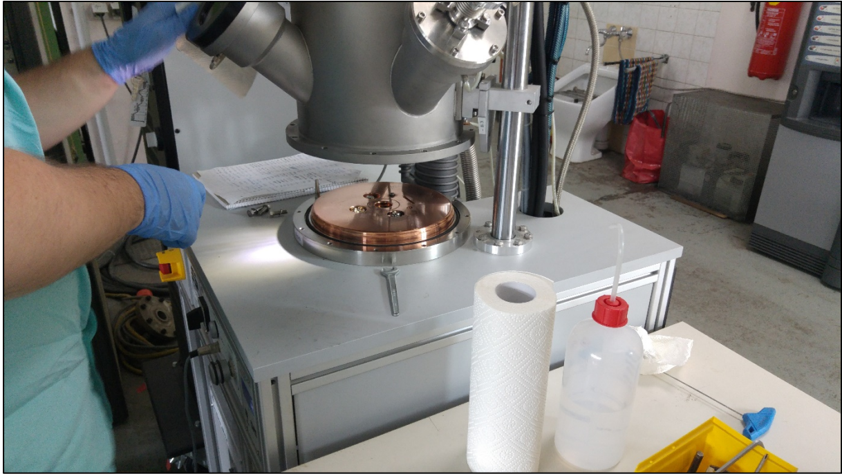
Figure 2.1: An image of the arc melter device used in this work.
