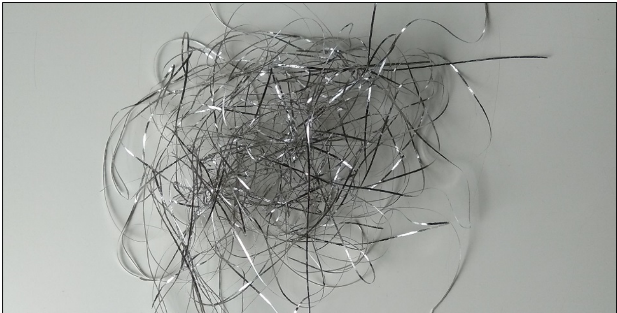
Figure 3.1: Overall view of MA-17 ( \text{Fe}_{80}\text{P}_{13}\text{C}_7 ) metallic glass ribbon.
