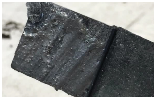
Figure 22: Metal layer formed on graphite cubes during the reduction of basic oxygen furnace slags in the InduMelt plant
