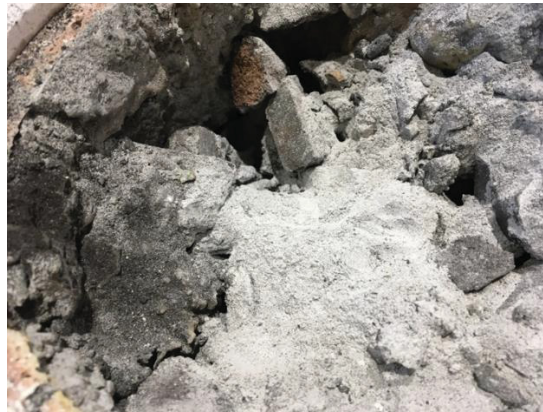
Figure 41: Powder found in the InduRed reactor after the second continuous experimental campaign
