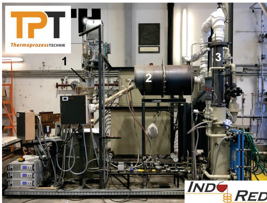
Figure 6: InduRed pilot-scale plant and its main components (1: reactor, 2: combustion chamber, 3: gas scrubber)
