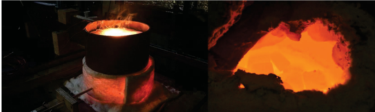
Figure 30: InduMelt plant during operation and heated graphite cubes shortly after tapping
