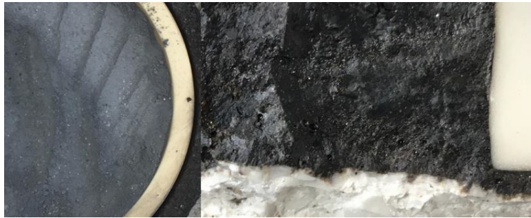
Figure 49: Synthetic slag mixture (left) and product after smelting (right) for reduction in the InduMelt plant
