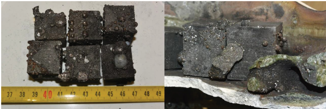
Figure 32: Complexity of metal and slag samples after reduction of basic oxygen furnace slags in the InduRed reactor (left: metal spheres on graphite cubes, right: metal on cubes and green, partially reduced product slag)
