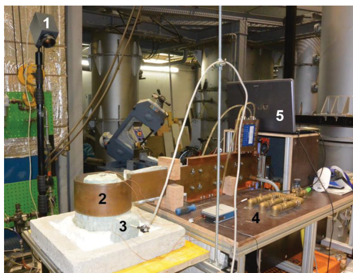
Figure 28: InduMelt plant and temperature measurement equipment in operation (1: optical temperature measurement, 2: induction coil with reactor, 3: thermocouples, 4: cooling water distribution, 5: laptop)
