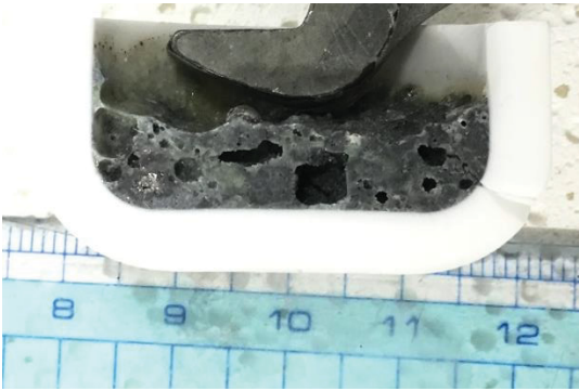
Figure 47: Metal and slag product phases after standard carbo-thermal reduction of Cr- and P-rich slag
