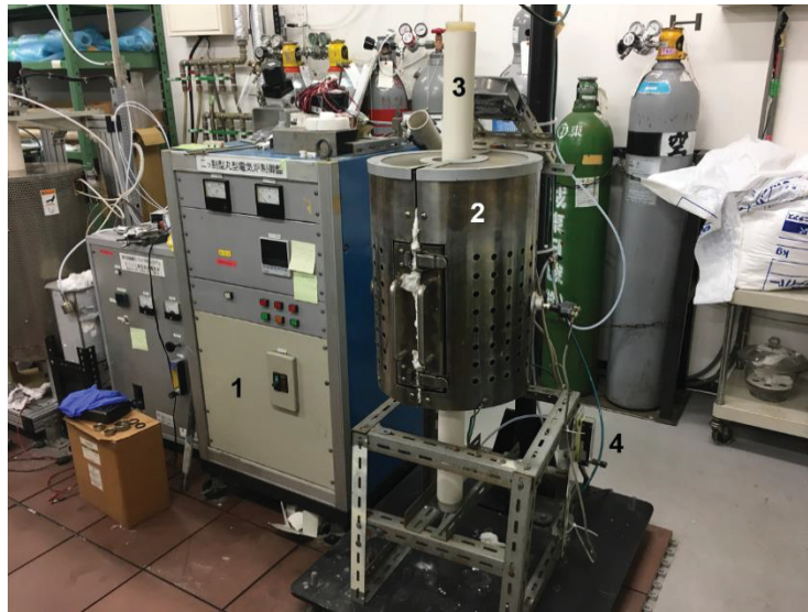
Figure 45: Furnace including equipment used for preliminary experiments with Cr- and P-rich slags at UTokyo (1: power supply and control unit, 2: furnace, 3: ceramics pipe holding the crucible, 4: Ar supply)
