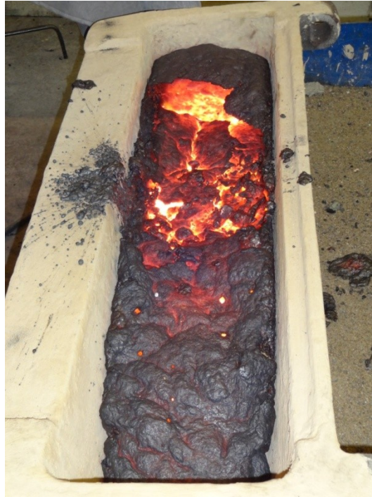
Figure 22: Slag on liquid iron bath in the mould
