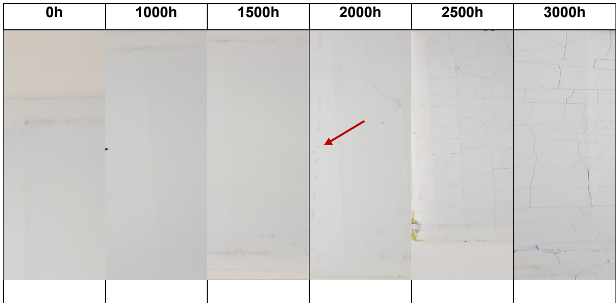
Figure 5.5. Cracking of the PET-laminate backsheet after tropical 2 test
