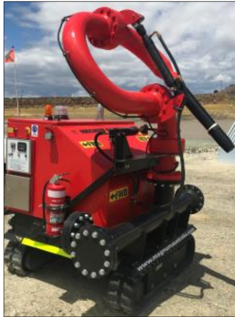
Figure 53. Hydraulic mining monitor (HR, 2019).
