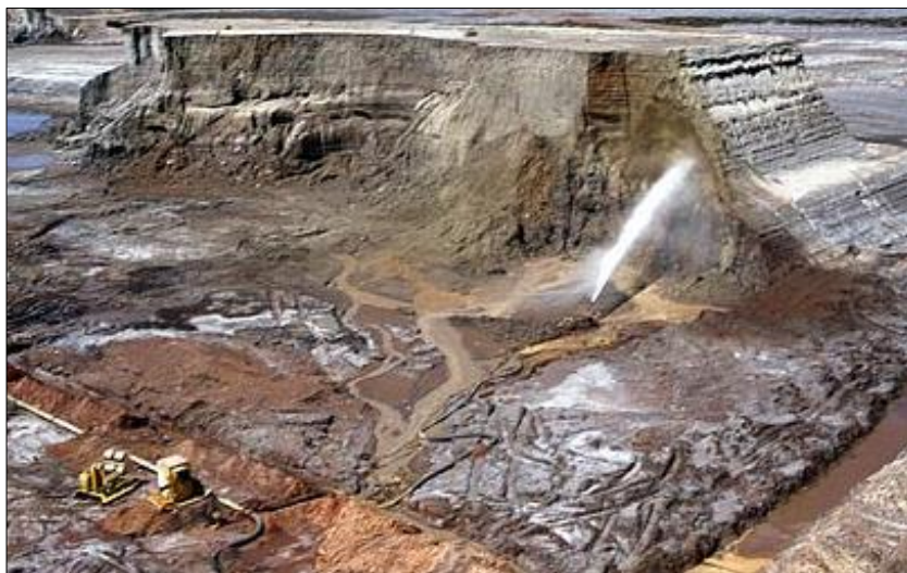
Figure 56. Hydraulic exploitation of tailings from the bottom (Engels, 2017).
