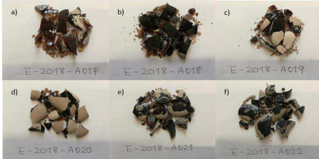
Figure 18. Quenched slags of a) A017, b) A018, c) A019, d) A020, e) A021, and f) A022.
