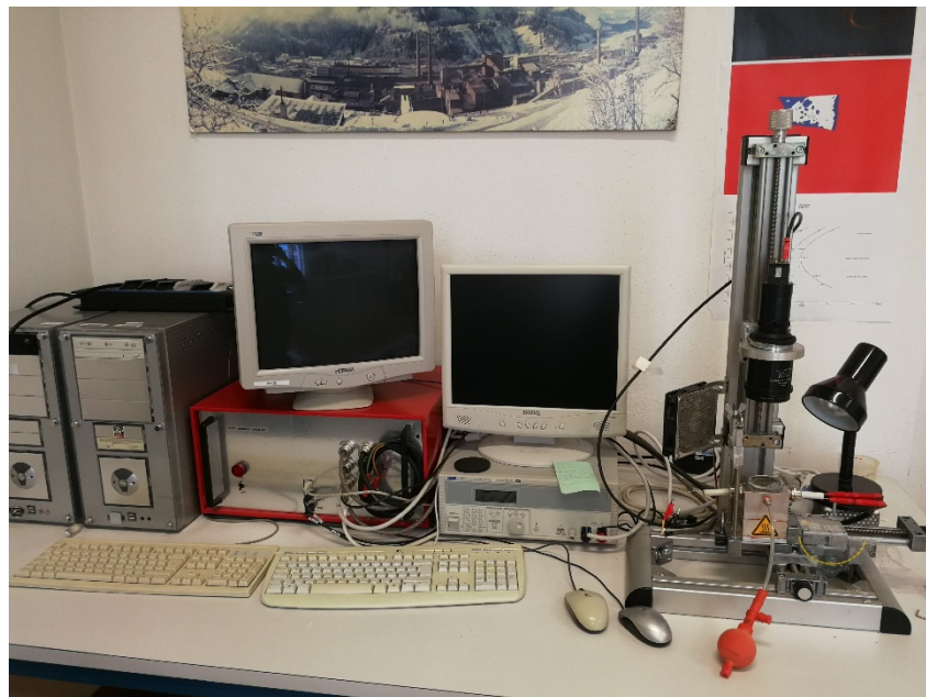
Figure 17: Single hot thermocouple technique equipment
