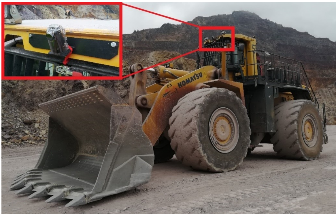
Figure 16: Loader with camera mounted on top of operator's cabin
