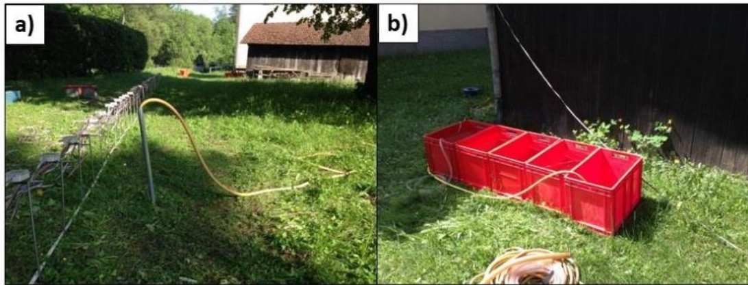
Fig. 27: (a) 1.0m deep well with garden hose at profile meter 15 for water introduction. (b) Containers for the provision of conductive (0.3 S/m) water.
