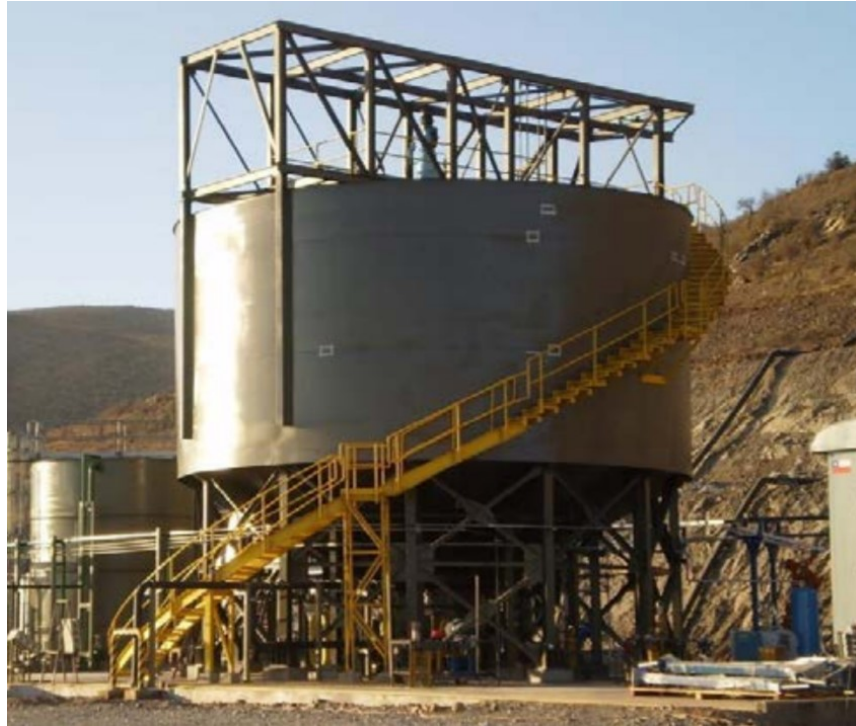
Figure 11: Typical deep cone thickener. Taken from Serbon, Mac-Namara, and Schoenbrunn (2016).
