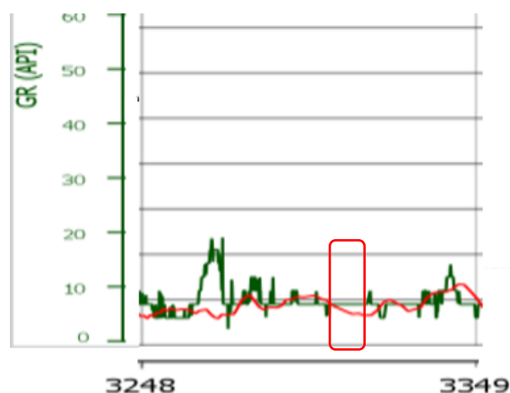
Figure 24. Example of a communication link malfunctioning.
