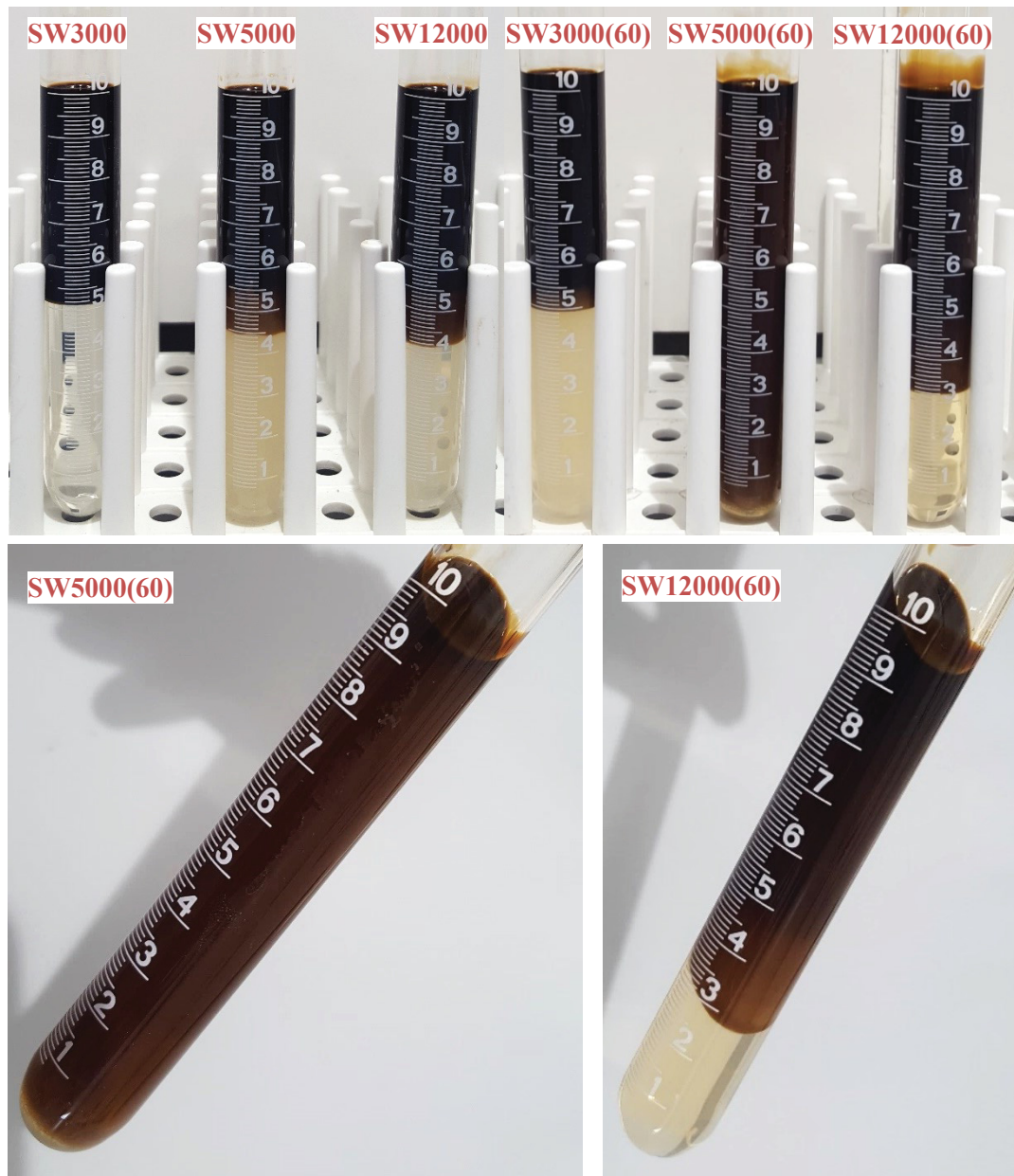
Figure 5.38 – Phase behaviour comparison at reservoir temperature conditions for 3000ppm to 12000ppm.
