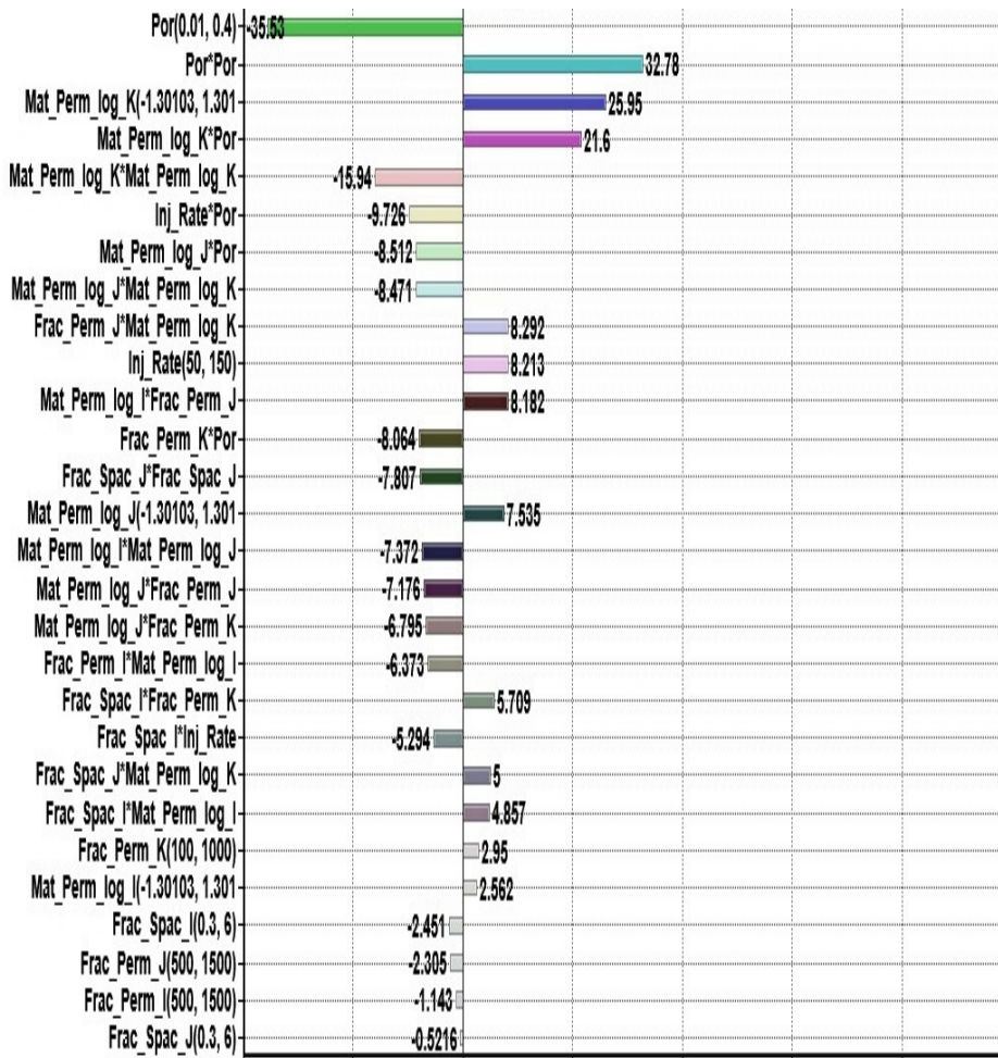
Figure 24 – Tornado plot shows the influences of each term on the recovery of Water Injection
