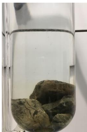
Figure 3. 50. Cavings in the extractor chamber.
