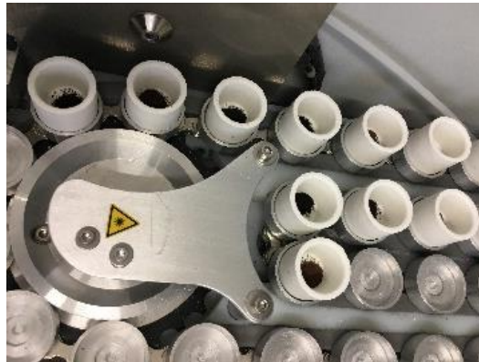
Figure 3. 51. Samples ready to be analyzed by the ELTRA Elemental Analyzer.
