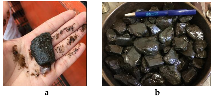
Figure 4. 1. Cavings collected at the drilling site, well S-6081. a) Showing one sample just taken from the shale shaker, b) All samples collected from the shale shaker.
