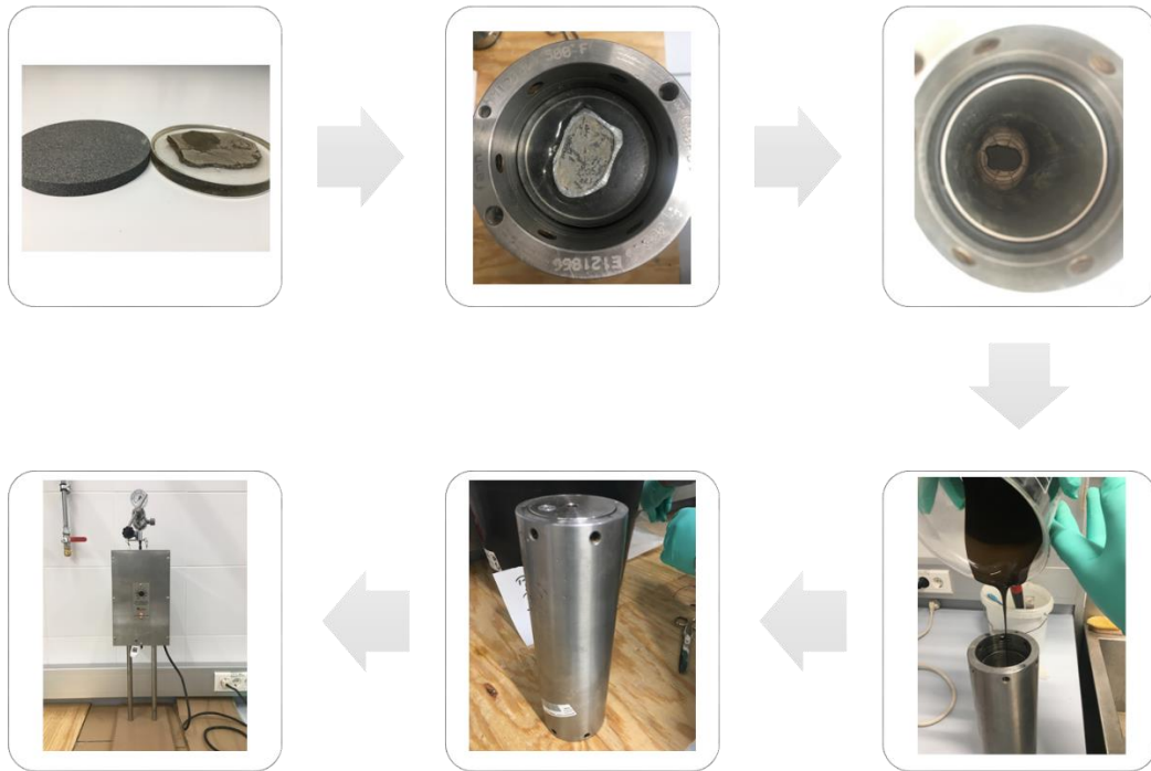
Figure 4. 5. HPHT Filter press test using disks made of epoxy and shale rock, and oil-base mud sample.
