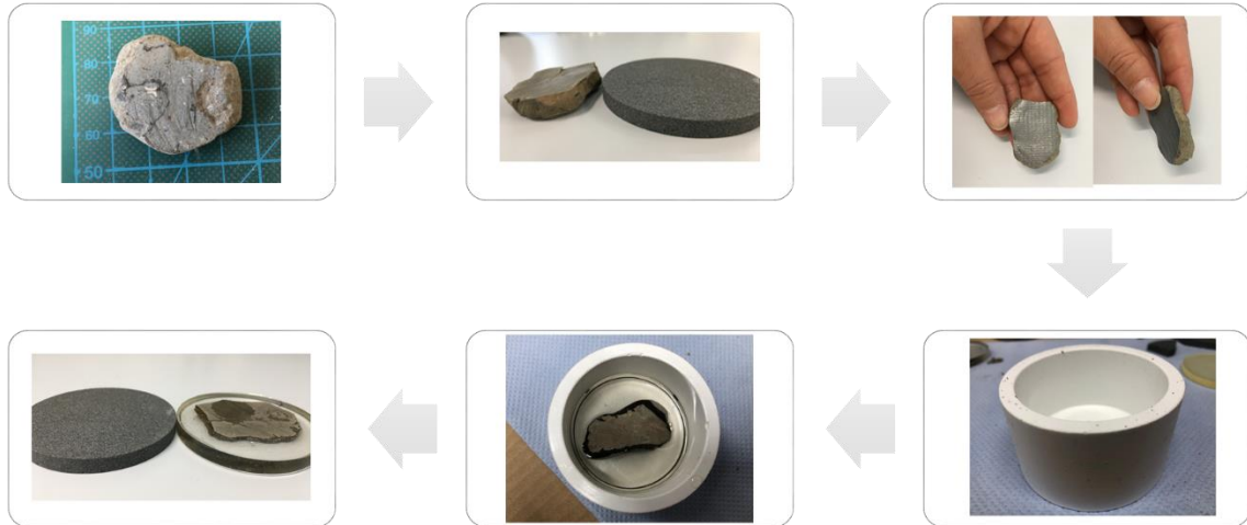
Figure 4. 4. Building procedure of the shale and epoxy disk to be tested.
