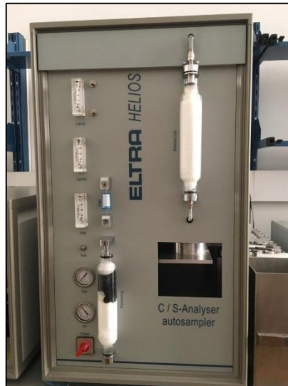
Figure 2. 3. Eltra CS-580A analyzer used to measure TC, S and TOC on shale samples placed at the Chair of Petroleum Geology.
