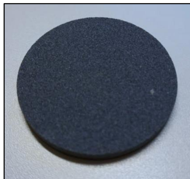
Figure 4. 3. Conventional ceramic disk used in the HP/HT filter press.
