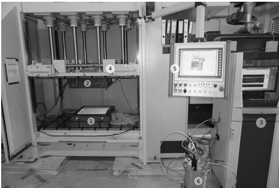
Figure 1 - The experimental setup. 1 - lower half of permeameter; 2 - upper half of permeameter; 3 - control panel for permeameter; 4 - hydraulic press; 5 - control panel for press; 6 - pressure pot; 7 - data acquisition system
