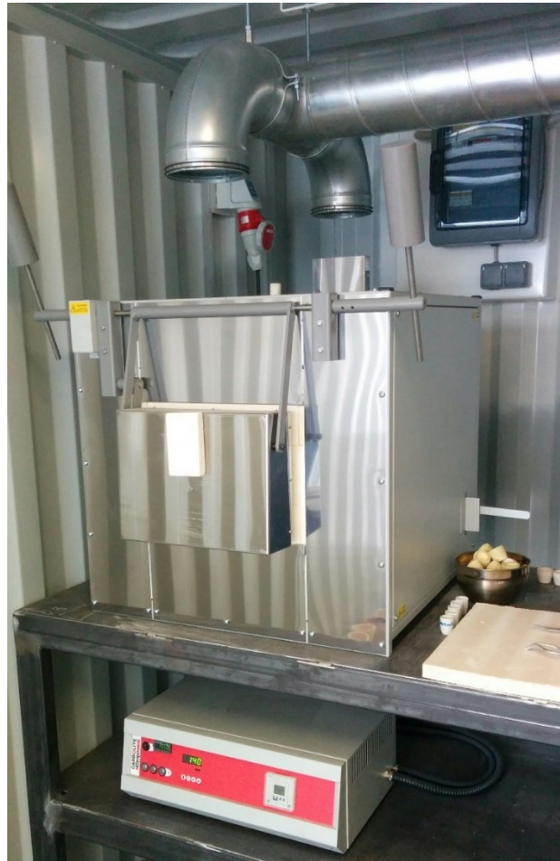
Abbildung 51: CF15 Cupellation Furnace – Firma Carbolite-Gero
