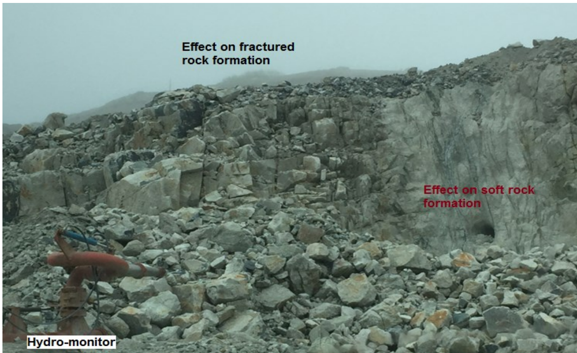
Figure 30: Effects of water jet on different rock formations (Horsley-Kozadjian, 2016)
