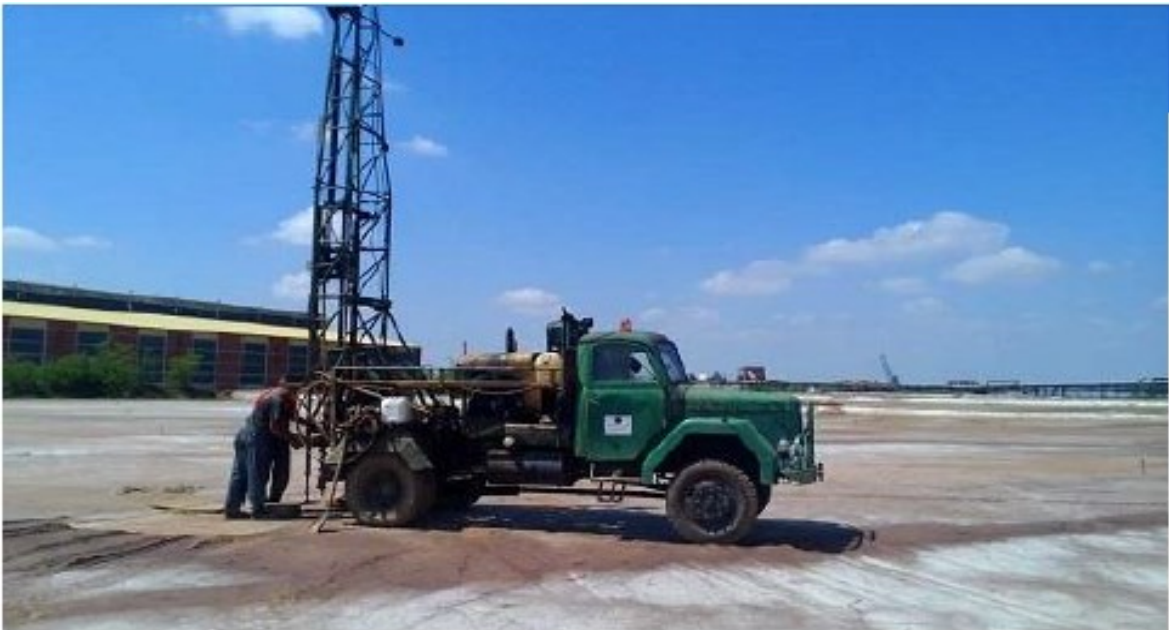
Figure 11: Producing samples from the dried surface of a jarosite pond (Elixir Group, 2013)
