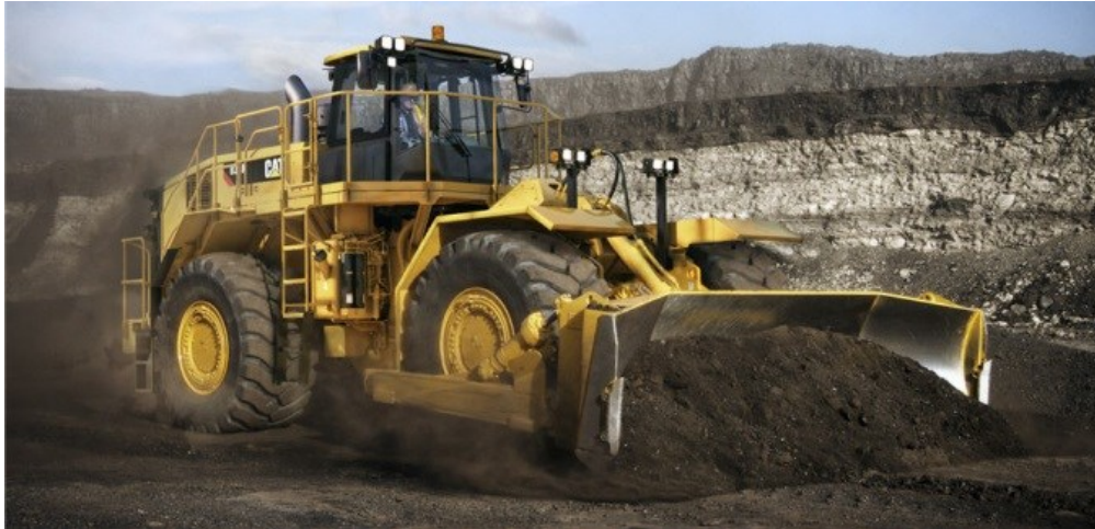
Figure 26: Dozer scraping material (Caterpillar, 2016)
