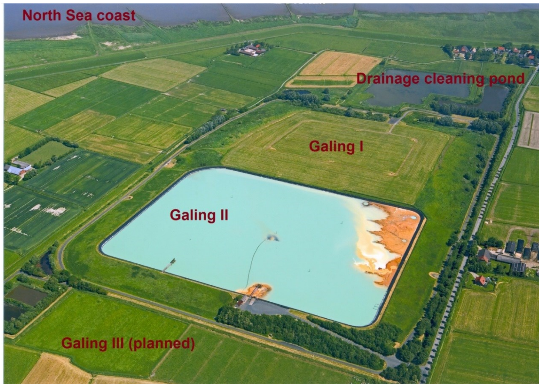
Figure 2: Jarosite slurry impoundments in Nordenham, Germany during filling (Galing II) and after renaturation has been completed (Galing I)
