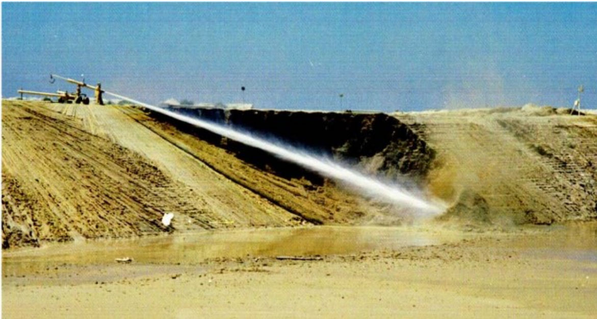
Figure 33: Hydraulic Mining of tailings with high pressure water jet establishing flat cutting angles (Roehl et al., 2007)
