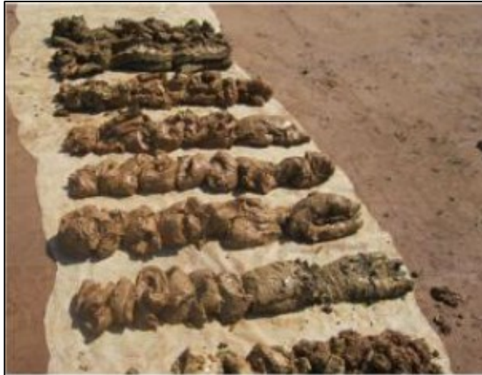
Figure 10: Drill cores produced from a jarosite impoundment (Elixir Group, 2013)
