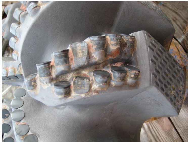
Fig. 2.15: Damaged cutters of a PDC bit. Some cutters have been sheared off or have parted from their matrix connection and are lost. (Baker Hughes 2015)
