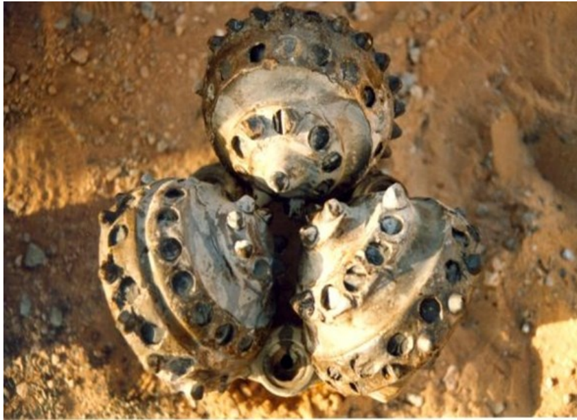
Fig. 2.13: Severely damaged cutting structure of a roller cone bit due to high axial vibrations. This can also lead to the total loss of one or more roller cones. (Baker Hughes 2015)
