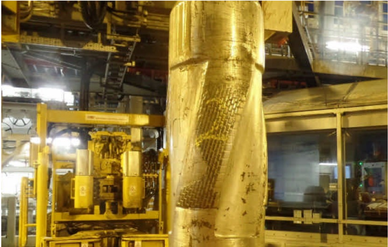
Fig. 2.18: Chipped-off tungsten-carbide inserts of a stabilizer blade due to high lateral vibrations. (Baker Hughes 2015)
