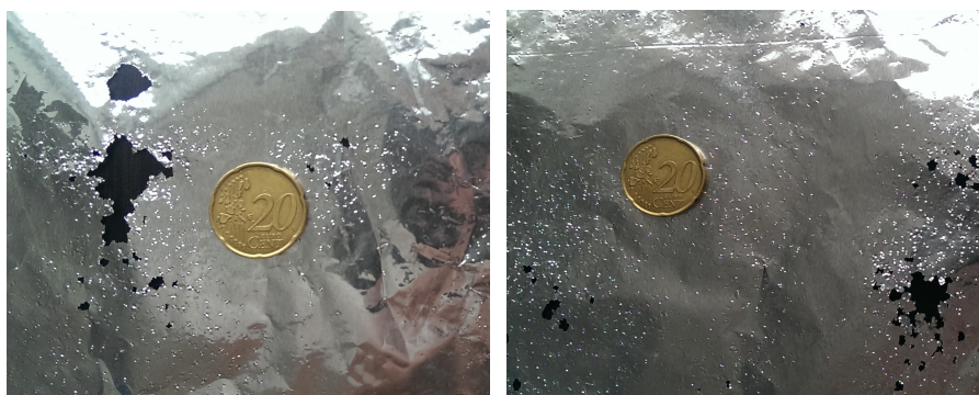
(a) Test, perforations directly pointing at the foil (b) Test, perforations with an angle to the foil
