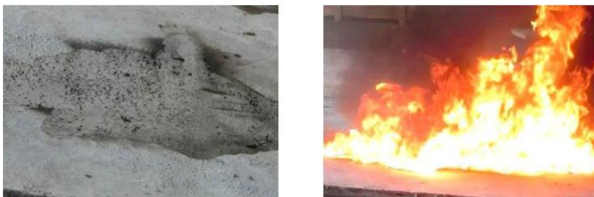
Figure 22: Pool of 0.6 l gasoline on concrete before and after ignition [8] p. 335
