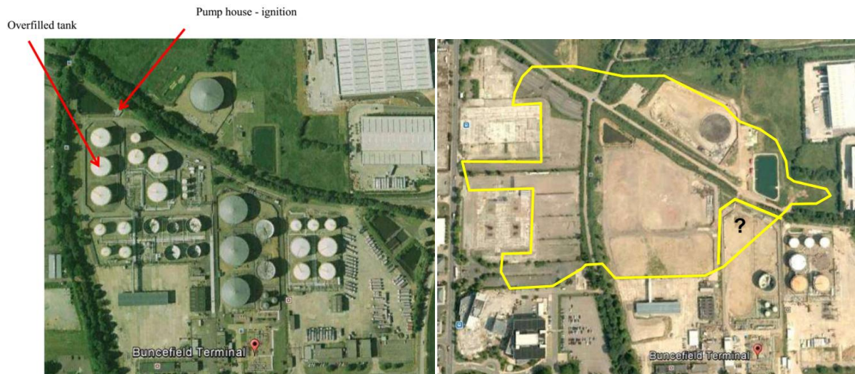
Figure 28: The site before and after the explosion, area of the vapour cloud marked [18] p. 49-50
