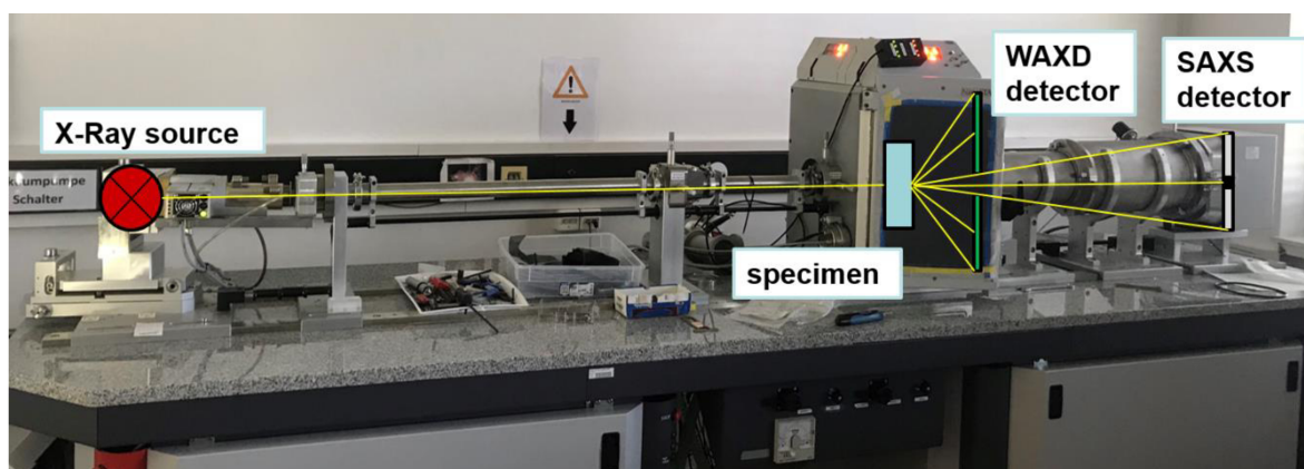
Fig. 3.11: Illustration of the Brucker NANOSTar used for the X-ray diffraction measurements.
