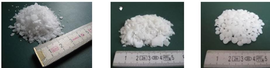
Abbildung 5: Links: LanXess AP Caprolactam Flakes; Mitte: Brüggemann Chemical Aktivator C20P; Rechts: Katalysator C10 [13].
