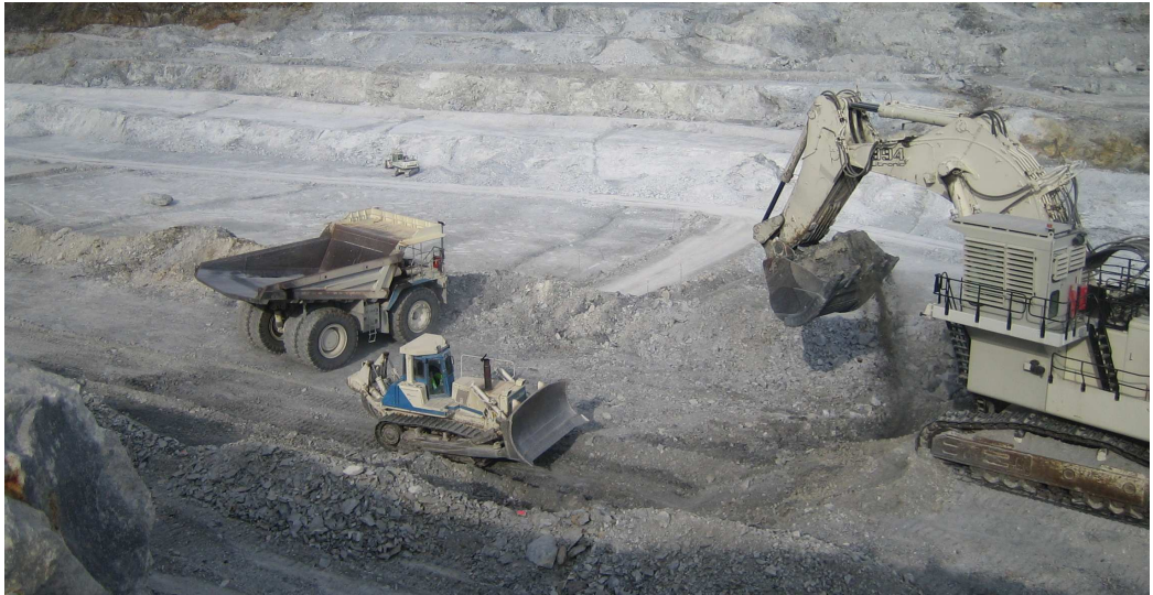
Figure 6.17: Dozer obstruct load and haul process due to limited space at load site
