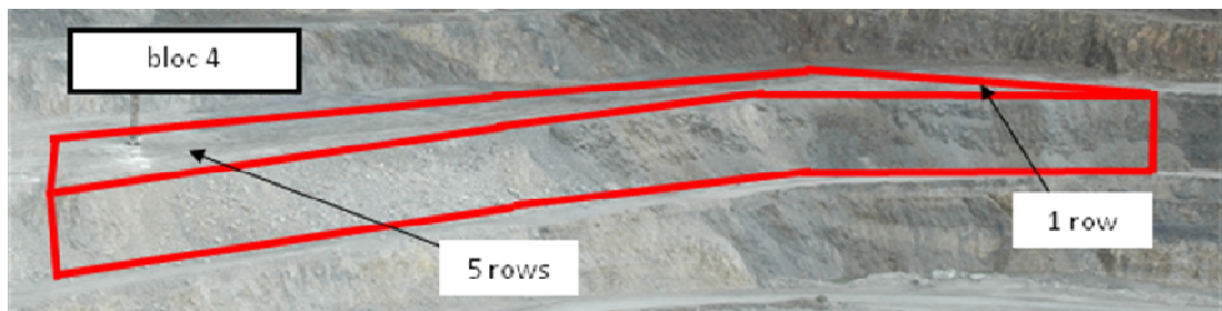
Figure 6.4: Single-row blasts at the end of bloc 4 , South
