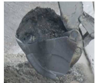
Figure 5.3: Example for used fill factor (fill factor 1 left, 2 middle and 3 right picture)
