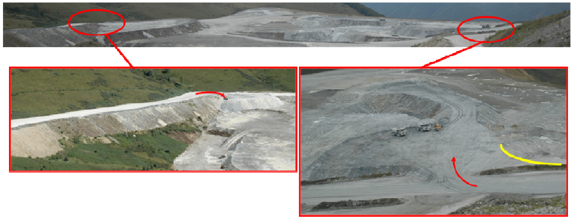
Figure 6.12: Narrow curves before loading on Vers Sud Nord (left) and Vers Sud Sud (right)
