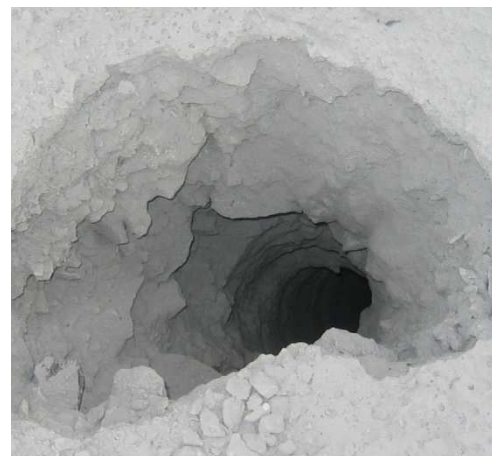
Figure 6.2: Borehole with increased diameter in schist (left) and with straight width in dolomite (right)
