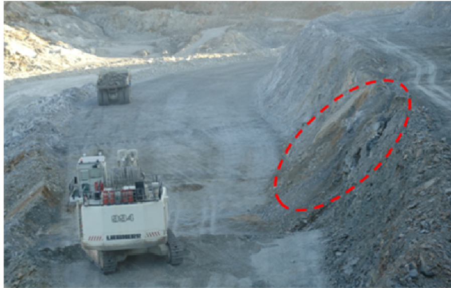
Figure 6.8: Rock fall after finishing loading and hauling, bloc 3
