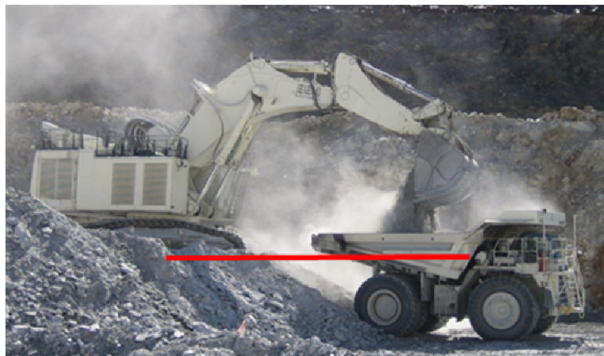
Figure 6.14: Low slice height on bloc 11 , slice 5
