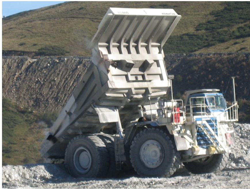
Figure 6.15: Discharging directly at the safety berm without waving in
