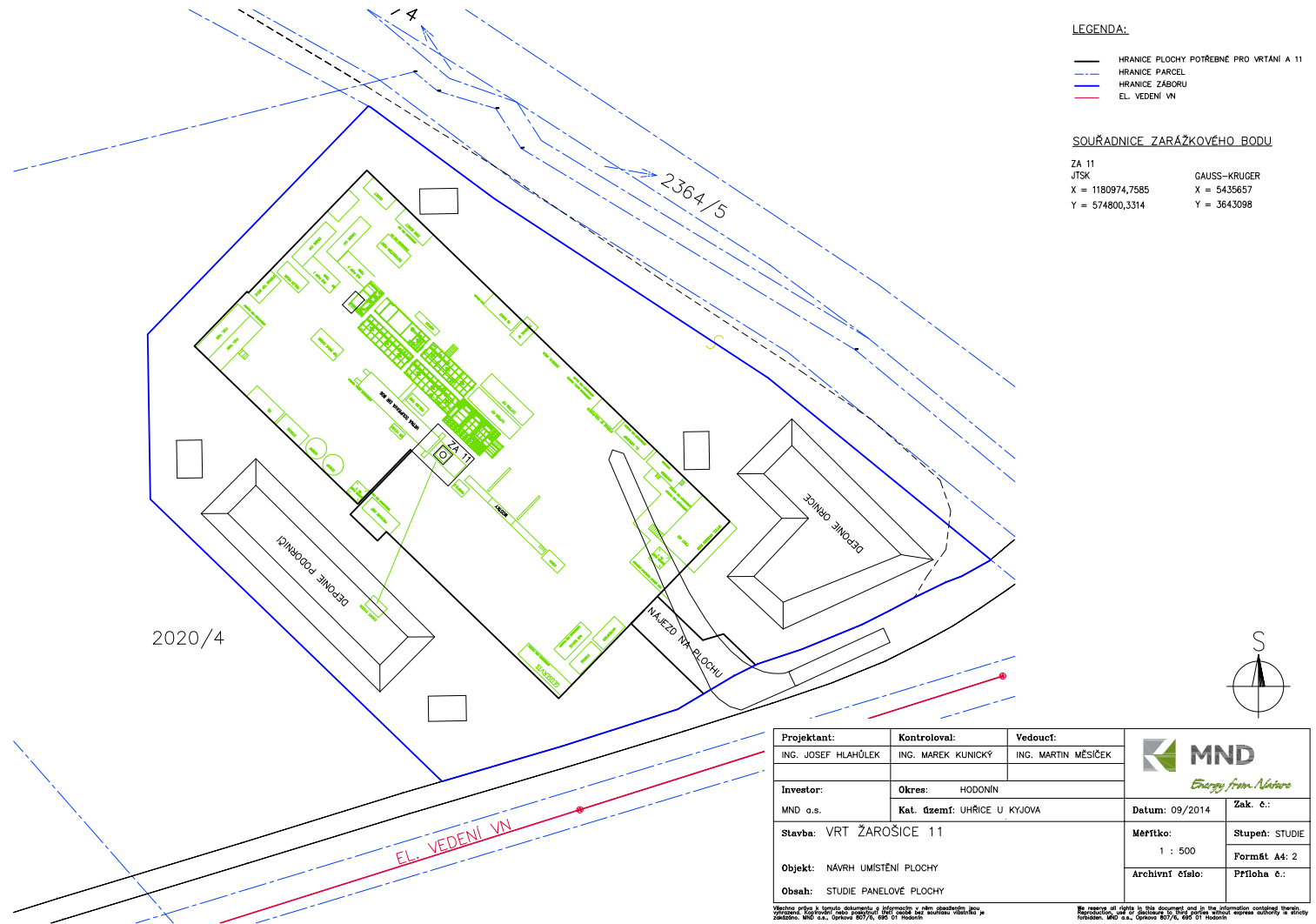
Figure 3.5.: Layout of ZA11 well site for a 150 t rig, which is anticipated by the operator. The inner area occupies an area of 3,200 m 2 which is more than double the required area of a LWDS rig.
