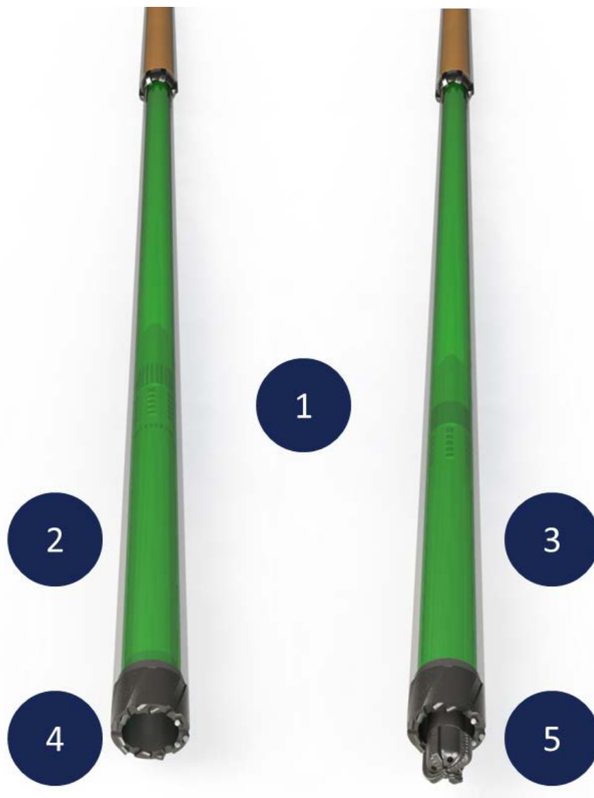
Figure 2.5.: Comparison of BHAs for full hole (right) and coring mode (left) of the LWDS. In full hole drilling mode the core barrel assembly is replaced by a drilling plug assembly that latches inside the SCD string. (1) latching and sealing assembly, (2) core barrel with bearing sections and core holder, (3) drilling BHA with optionally PDM, measurement tools and other tools, (4) rim bit only, for coring mode, (5) full hole mode with rim and pilot bit. Schematic illustration only. Not to scale.
