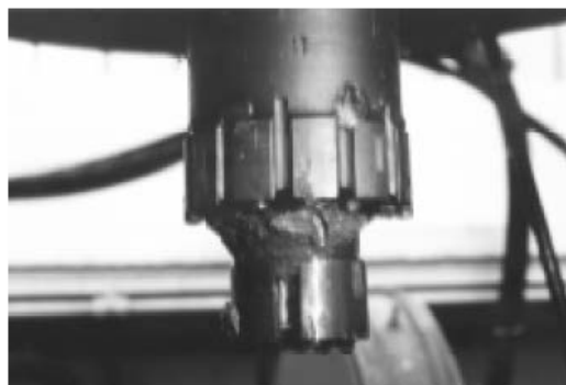
Fig. 4- Bit balling occurred at the corner between the drill plug and core bit (rim).
