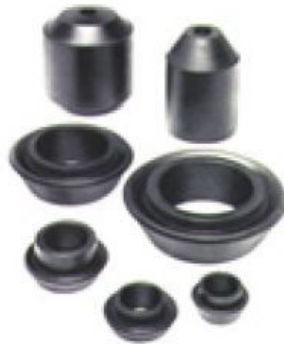
Figure 25: A variety of swab cups. The aim is, that the cup dives into the liquid and pushes it upwards when the cups are retrieved to surface via wireline.
