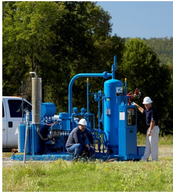
Figure 35: CSI Compresso GasJack system, and how it is utilized in the US [38]
