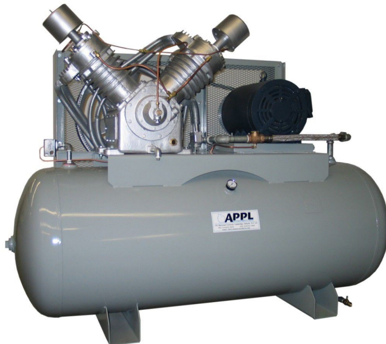
Figure 7: Small industrial air compressor (~25 HP) 13
