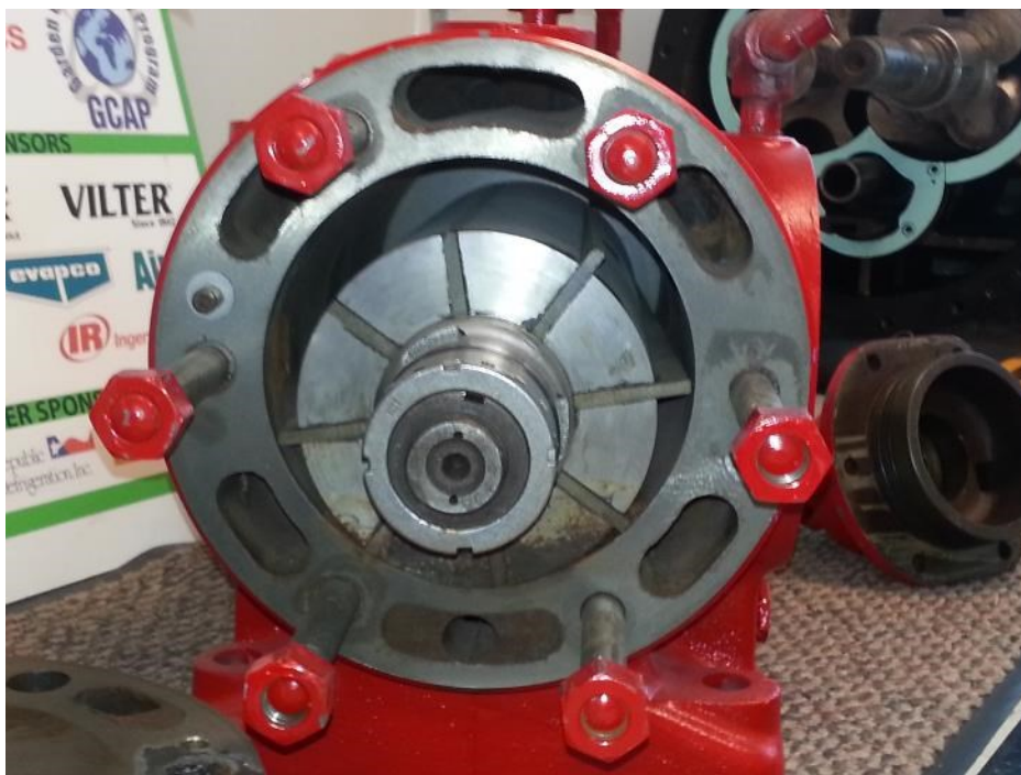
Figure 15: Opened ammonia compressor incorporating eight vanes 24
