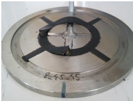
(a) Stuck and fractured part in the fixed side
