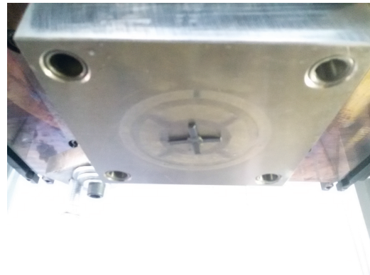
(b) Stuck and fractured runner in the moving side
