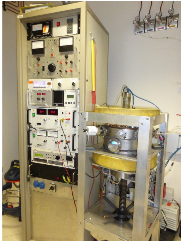
Figure 3.1: Magnetron sputter deposition system “Margot”.
