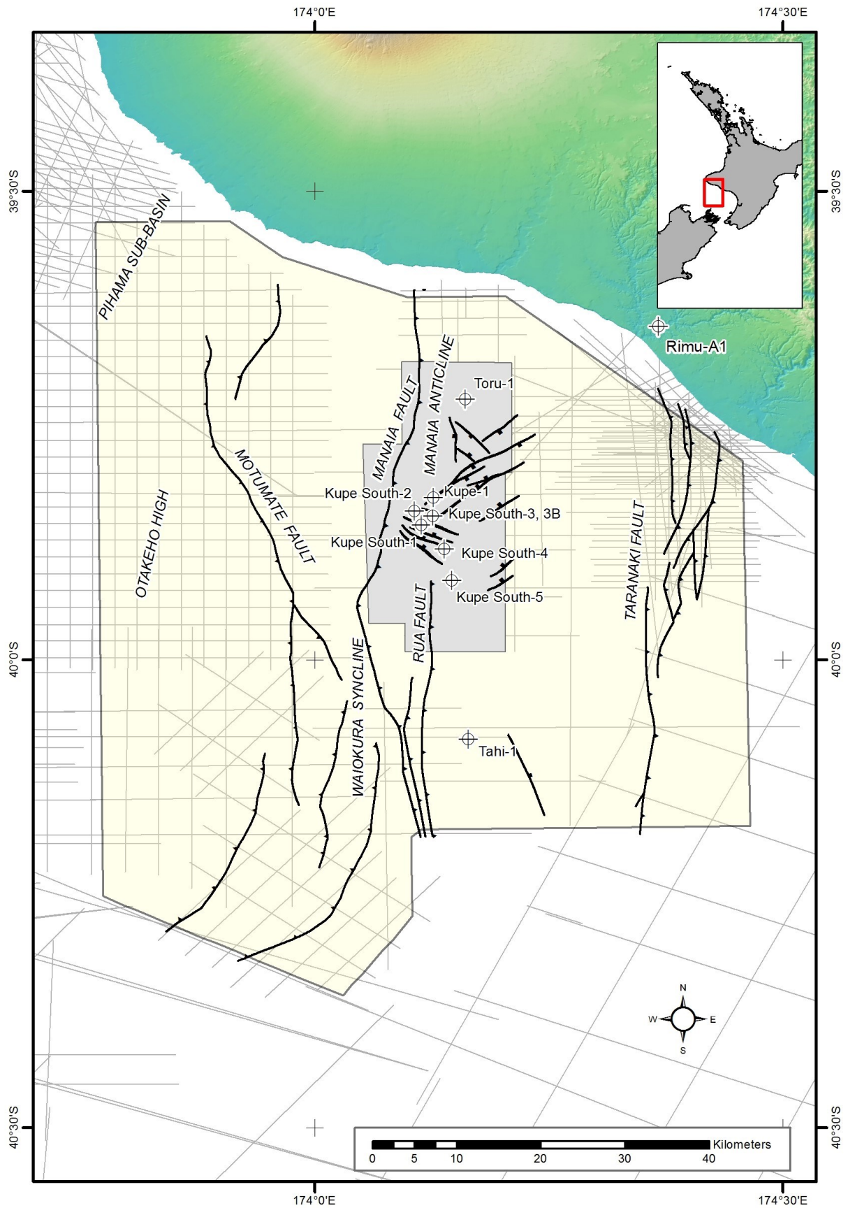
Figure 6: Schematic map of the KUP area (yellow polygon) with seismic cube Kerry 3D (grey polygon), 2D seismic lines (grey lines), well locations (circles) and main structural features (black lines) (Fohrmann et al., 2012).
