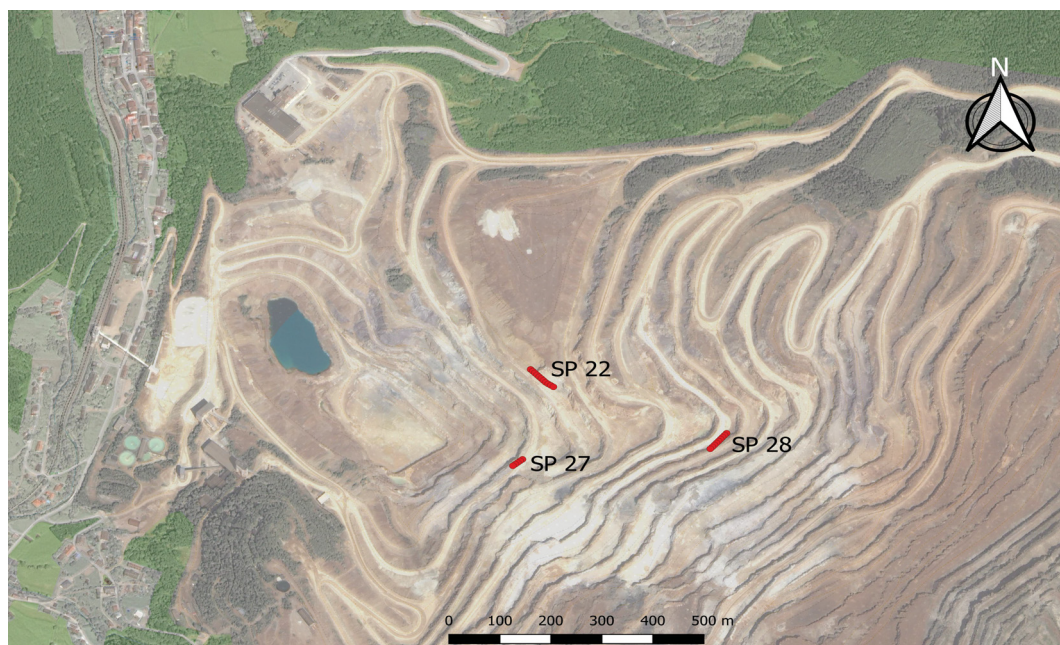
Figure 4.3: Borehole configuration for SP 22 (SYBO298), SP 27 (ETM3371) and SP 28 (PALM385)
