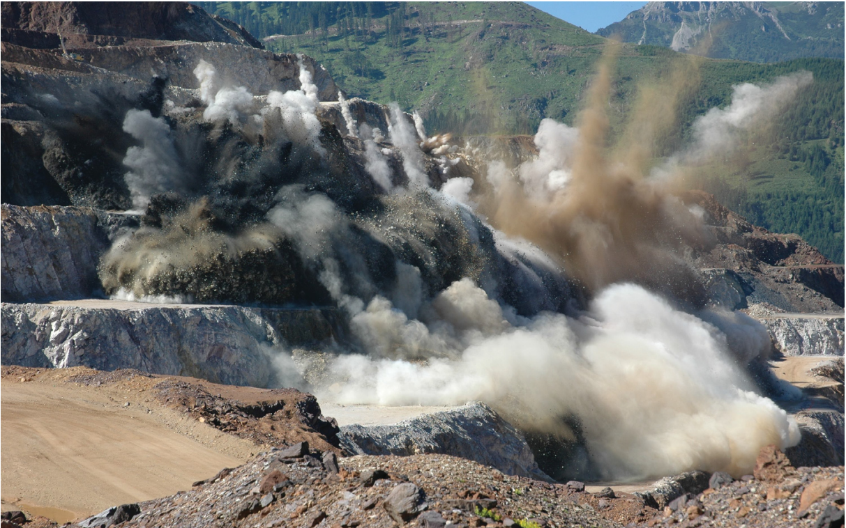
Figure 1.1: Example of a production detonation at Mt. Erzberg mine ( http://www.vaerzberg.at/ , retrieved August 19, 2018)
