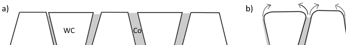
Fig. 8: Scheme of a) the cemented carbide substrate after polishing and b) the polished cemented carbide substrate after ion etching. The arrows indicate the removal of material by Ar ion etching.
