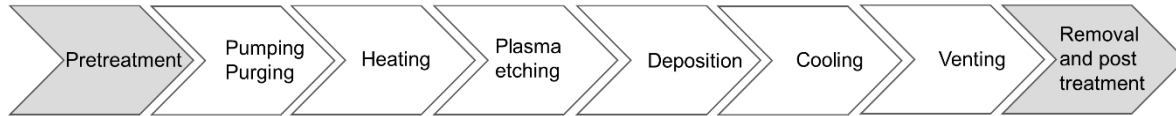
Fig. 1: Sequential steps of deposition processes. In the case of the PVD processes, the steps Pumping, Purging and Venting have been included into the steps Heating and Cooling, respectively. In the case of the CVD process, the step Pumping/Purging was included into the step Heating; the steps Plasma etching and Venting are absent.
