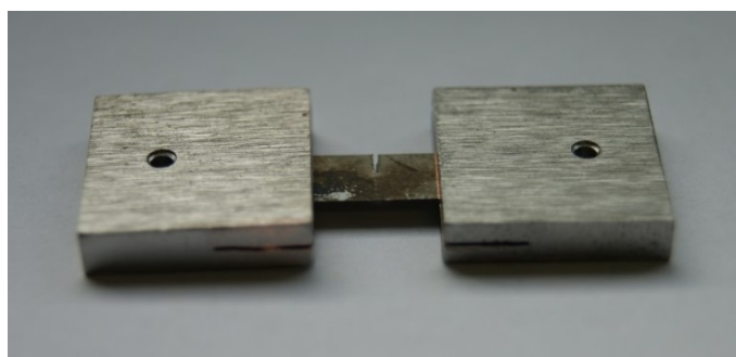
Figure A.3. Fracture experiment sample, tungsten foil pre – cracked with diamond wire saw, razor blade and FIB and then brazed between two steel holders.
