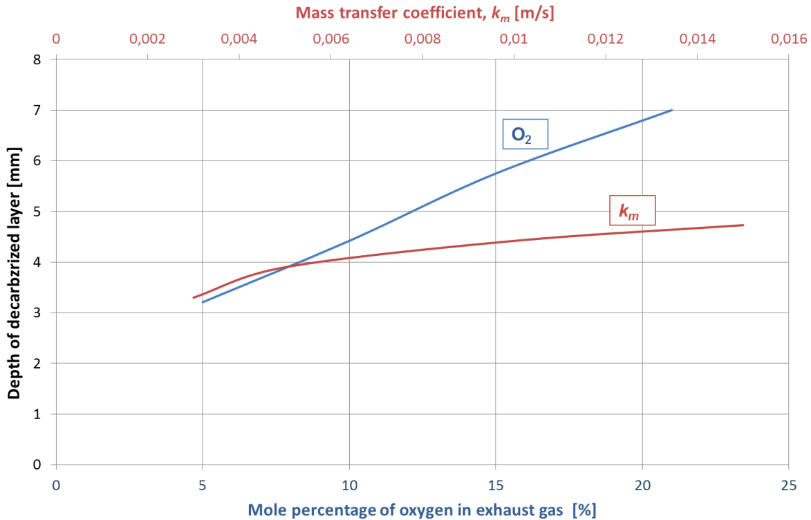
Fig. 57: Comparison of two parameters influencing the depth of decarburized layer in MgO-C refractory
