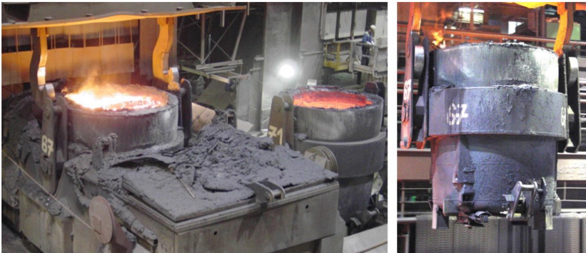
Fig. 7: Steel ladle during service: a) at the left side filled ladle will be just taken by a crane, at the right side empty ladle; b) ladle transported by a crane [62].
