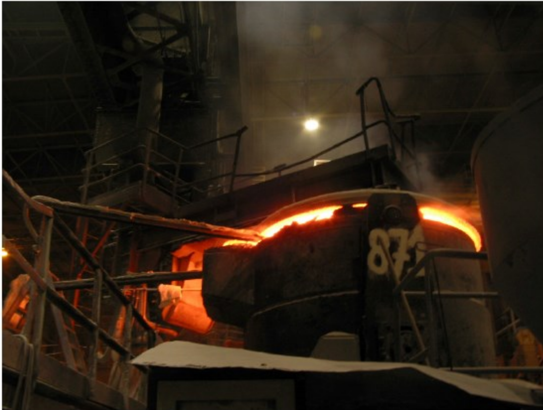
Fig. 8: Photographic representation of a ladle preheating station [65]
