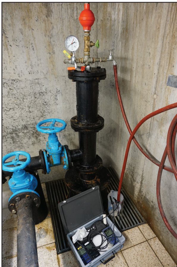
FIGURE 5.1: Measurement of field parameters (Temperature, pH, Conductivity and Eh) at a sampling site (courtesy of Łukasz Pytlak)
