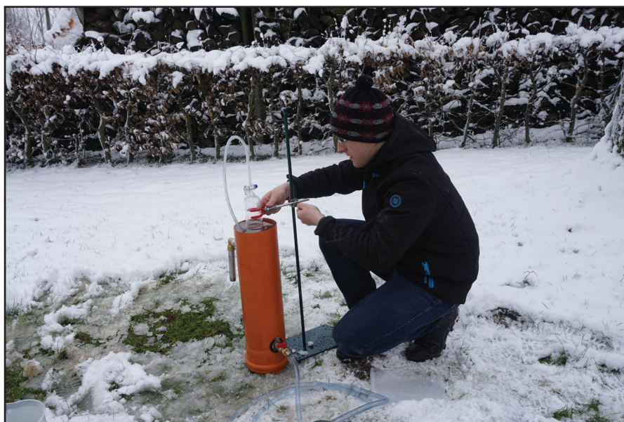
FIGURE 5.2: Gas sampling with a sampling device developed by Łukasz Pytlak (courtesy of Łukasz Pytlak)
