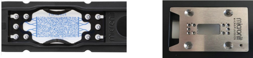
Figure 3-6- Physical rock micromodel in left and High-Pressure chip holder in right (Micronit, 2018)
