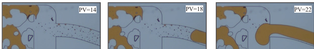
Figure 5-7- Oil entering micromodel during waterflooding, time steps is from left to right
