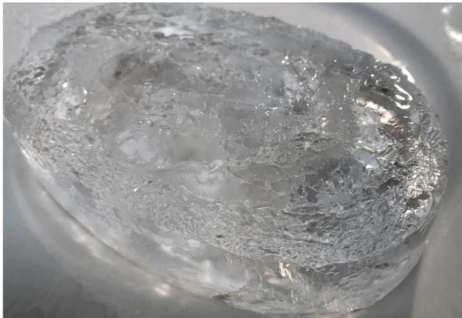
Figure 39: Ice after 10 minutes of ultrasonic excitation. Ice disintegrates in form of blocky breakouts. Very brittle at the bottom.
