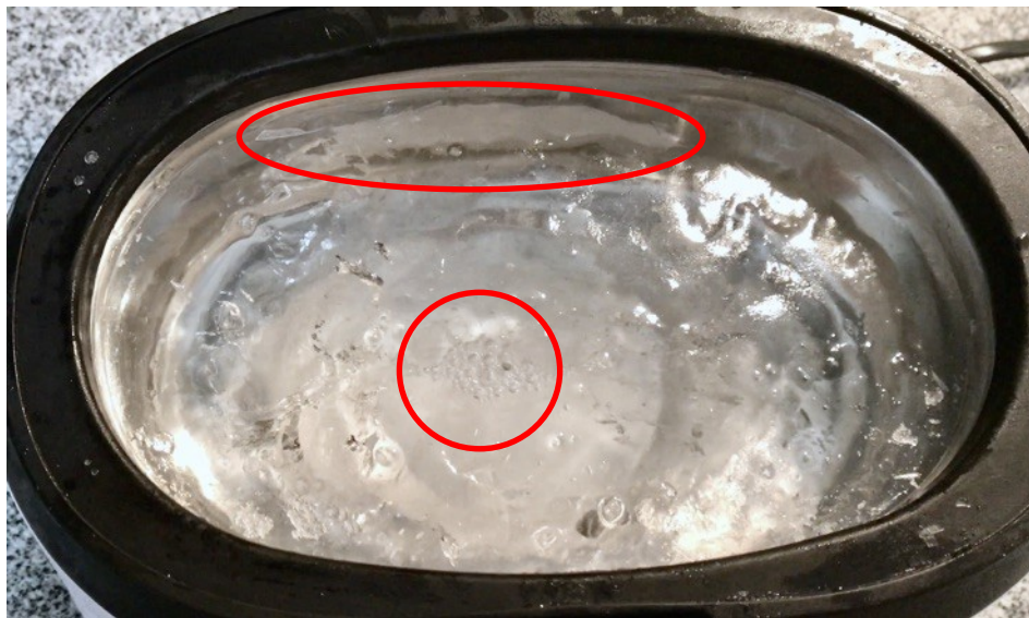
Figure 37: Block of ice after 4 seconds of ultrasonic excitation. Red circles indicate air bubbles due to cavitation effects.
