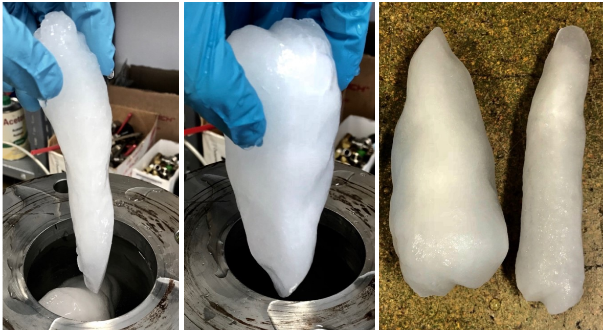
Figure 43: Remaining inner ice core after 160 minutes of ultrasonic excitation.
