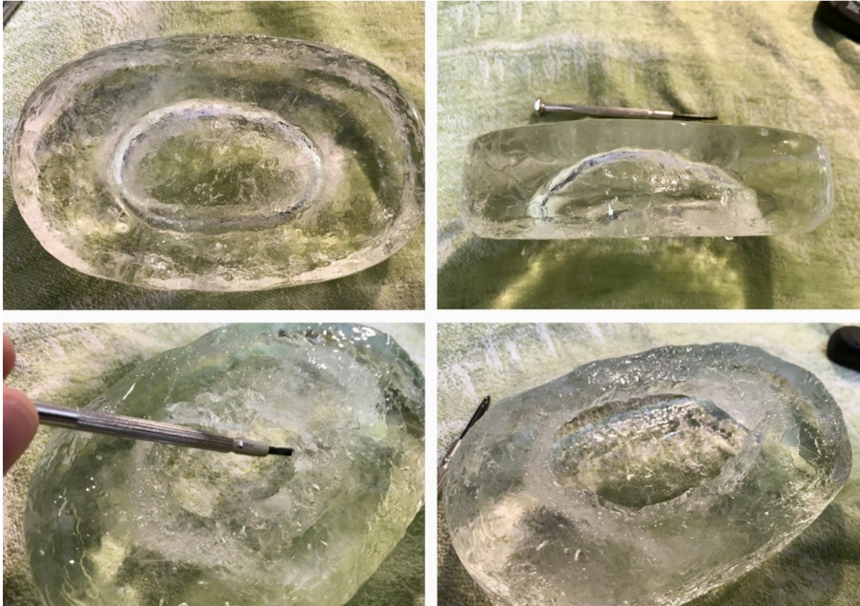
Figure 40: Block of ice after 20 minutes of ultrasonic excitation. A cavity as an effect of ultrasonic cavitation is seen.
