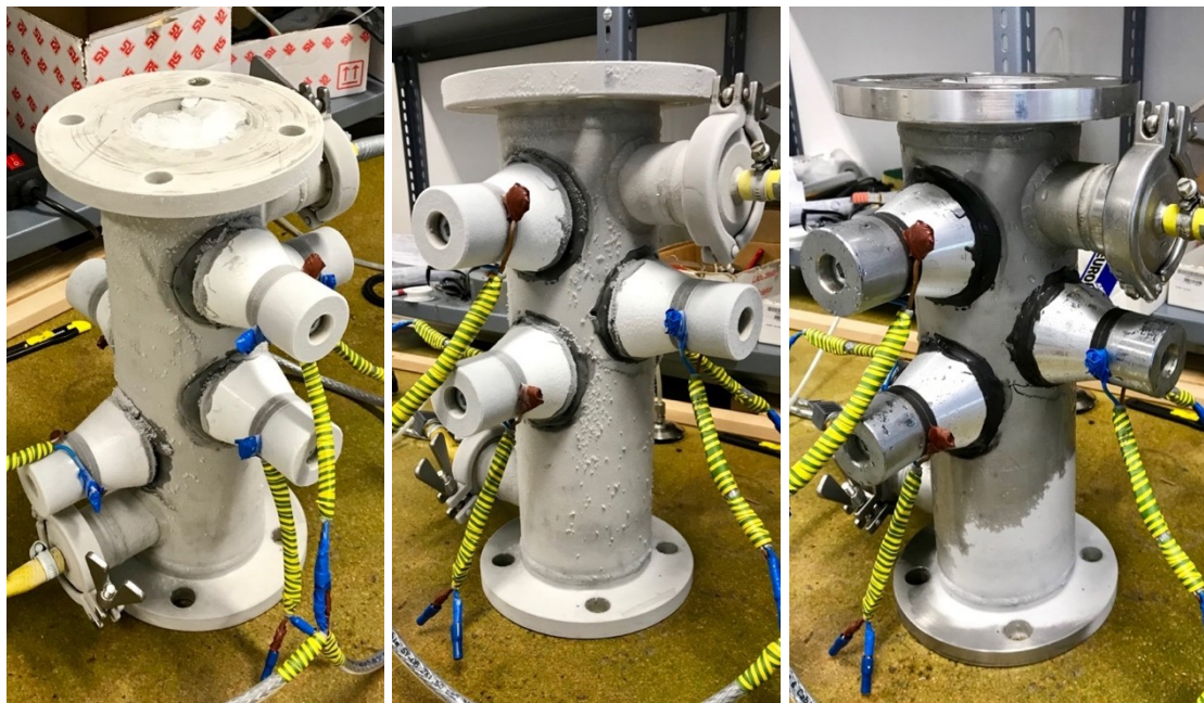
Figure 35: Steel cylinder after 0, 5 and 40 minutes of ultrasonic excitation.
