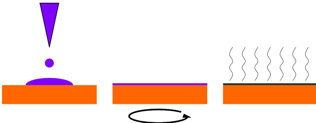
Figure 4: Schematic representation of the spin-coating process: A liquid precursor solution is dropped on the substrate (left). A thin layer of the liquid solution is formed by rotation (center), which is transformed into an oxide film by thermal annealing (right).
