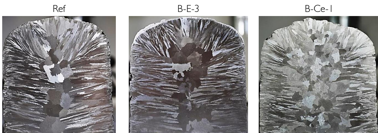
Figure 5-14: Examples for macrostructures with and without grain refinement – Series B
