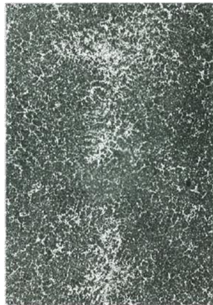
Figure 3-9: Carbide clusters through inhomogeneous distribution of nucleation sites (x20) [99]
