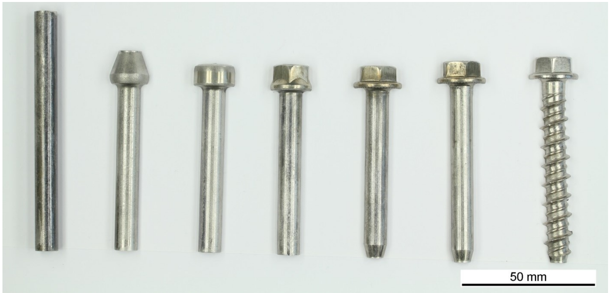
Fig. 3-4: Geometry of the HUS-HR 10x65 after each forming step and after thread rolling.
