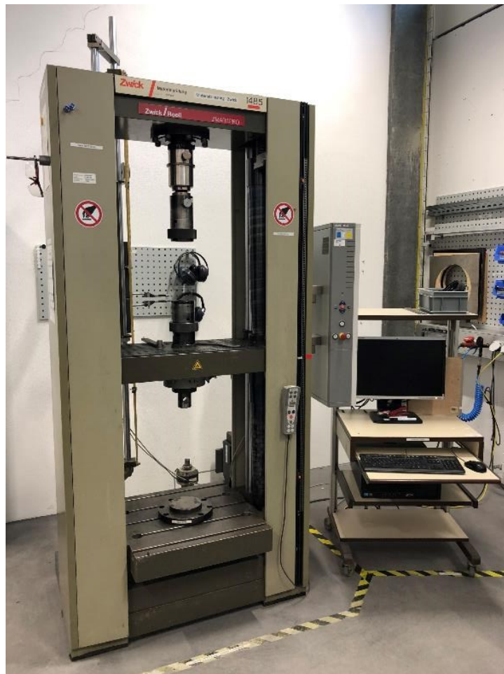
Fig. 3-5: UPM Zwick & Roell “Zwick 1485” used for the crush tests at Hilti AG.
