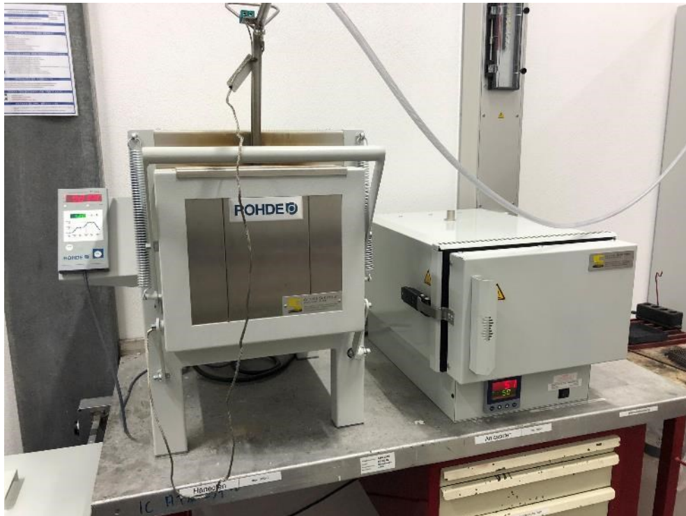
Fig. 3-7: Chamber furnace used to heat the samples for crush tests.
