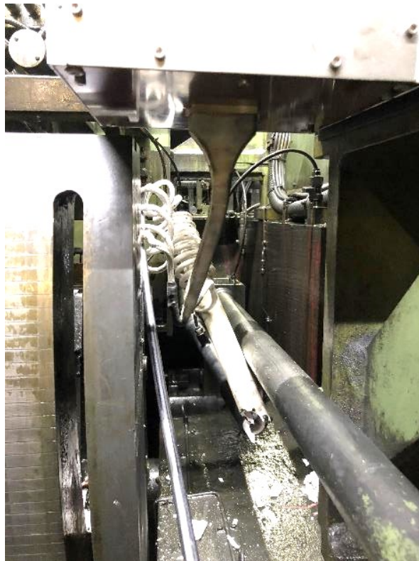
Fig. 4-3: The crash after the malfunction of the inductor control leading to a failure of the ceramic tube and the inductor.
