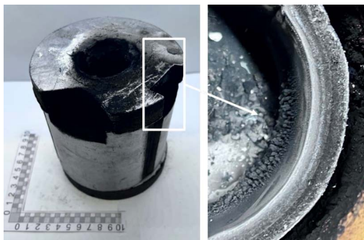
Figure 47. The reaction chamber following the test, showing carbon deposited on its inner surface [92] .
