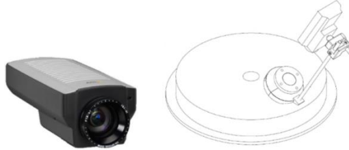
Figure 45. The camera system and instalment to the top lid of the plasma furnace [92] .
