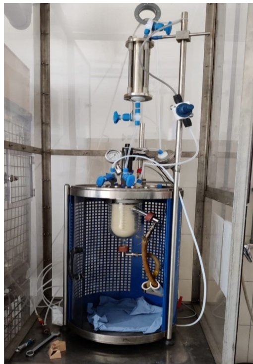
Figure 27: Construction of the autoclave used in the experiments
