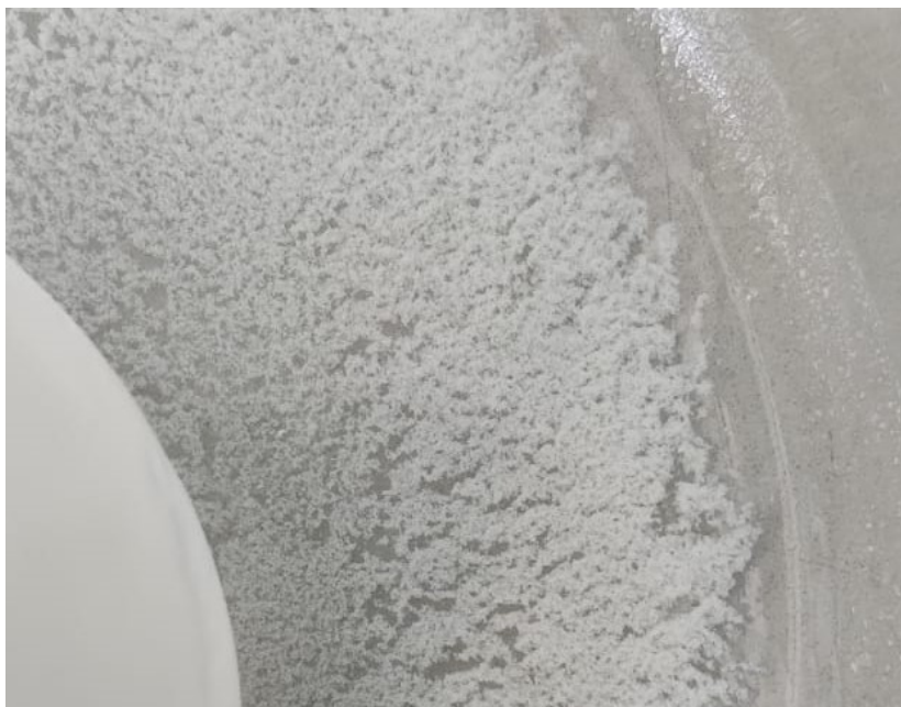
Figure 35: Appearance of the precipitate after addition of (\text{NH}_4)_2\text{SO}_4
