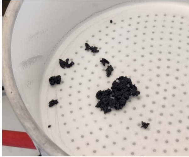
Figure 34: Solid residue of the filtration step after the cementation of lead
