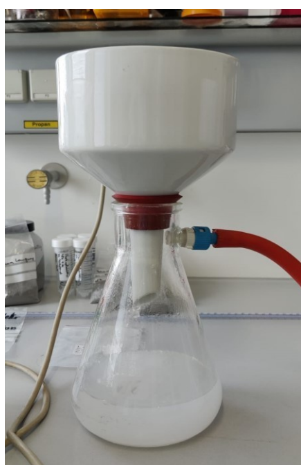
Figure 6: Experimental setup during the filtration of the solution (left), dried iron filtration cake (right)
