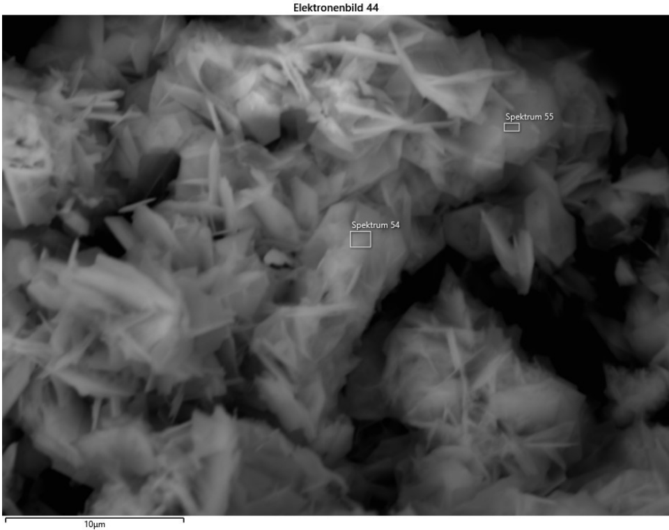
Figure 42: SEM picture of the zinc precipitate from the original route without treatment
