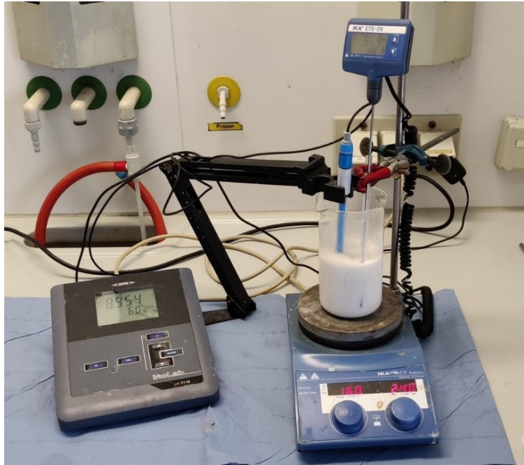
Figure 25: Experimental setup for the Soda leaching experiments on the example of the 60 °C experiment
